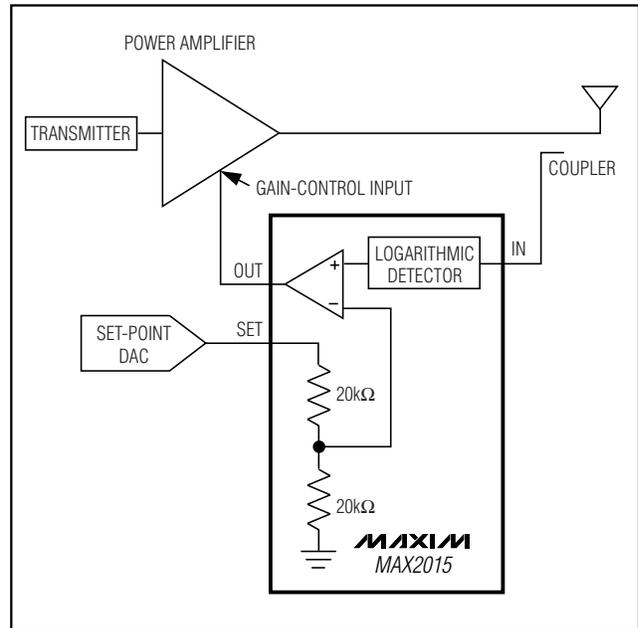
Figure 3. System Diagram for Automatic Gain-Control Loop
