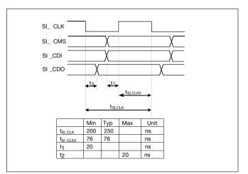
Figure 7. Timing diagram of the serial interface.
