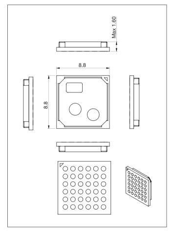
Figure 9. Mechanical dimensions and footprint
