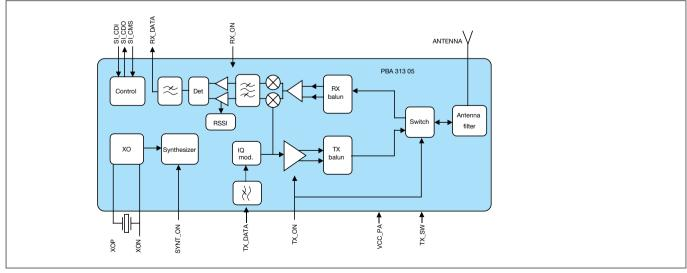
Figure 4. PBA 313 05 block diagram
