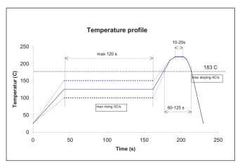
Figure 8. Eutectic SnPb-solder profile.
