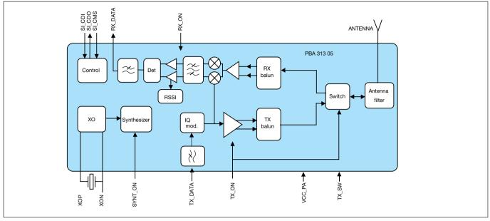
Figure 1. Block diagram.
