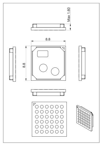
Figure 3. Mechanical dimensions and footprint.
