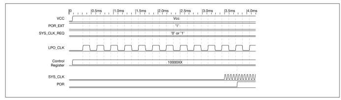
Figure 6. Powering up the module.
