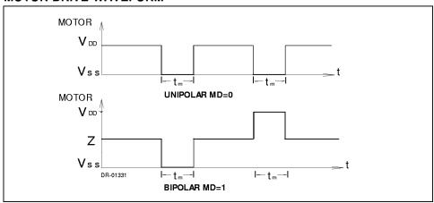
The pulse width for  $t_{\scriptscriptstyle m}$  is selected by the status of the motor pulse width input pin, MPW. The two possible options are shown in the following table.
