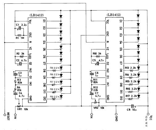
Note: Input signal of approximately 110 mVrms causes D8 (0 dB display) to light.
