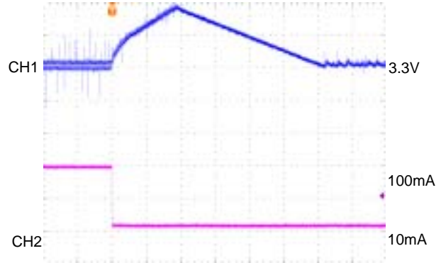
200usec/div CH1:V OUT1 , AC-COUPLED, 50mV/div CH2:I OUT1 , 50mA/div
