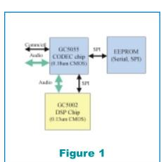
cores and high performance hard-wired co-processors. It provides extensive computational capability without compromising battery life. The unique architecture of the GC5002 simultaneously offers the flexibility of a programmable platform and the performance of hard-wired design. The chip utilizes a distributed and re-configurable architecture which enables hardware scalability and ensures
