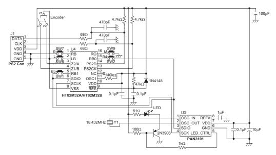
HT82M32A/HT82M32B Z-Axis Optomechanical (This Application Circuit is for Reference Only)
