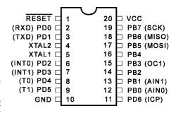
B output buffers can sink 20mA and can drive LED displays directly. When pins PB0 to PB7 are used as inputs and are externally pulled low, they will source current if the internal pull-up resistors are activated. Port B also serves the functions of various special features of the IN90S2313 as listed on page 38.
