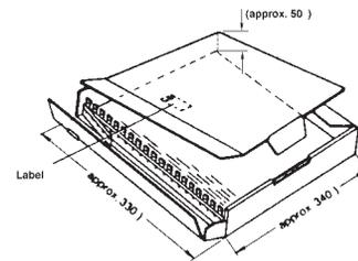
**Taping Dimensions for MKT 050 Series (5mm Pitch)**
