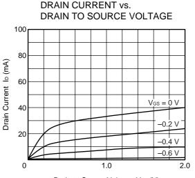
Drain to Source Voltage VDS (V)
