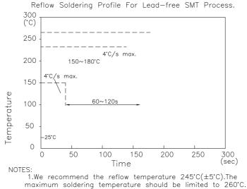
2.Don't cause stress to the epoxy resin while it is exposed to high temperature.
