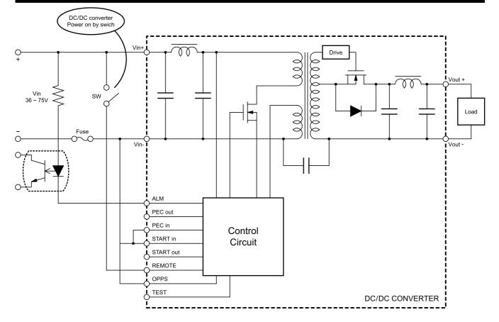
\* Please connect from PECin PIN, STARTin PIN, OPPS PIN to Vin-PIN in Natural Convection.
