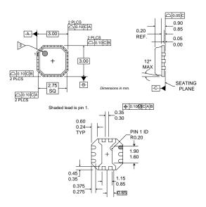
Package Style: QFN, 12-Pin, 3x3
