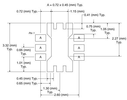
Figure 2. PCB Solder Mask (Top View)
