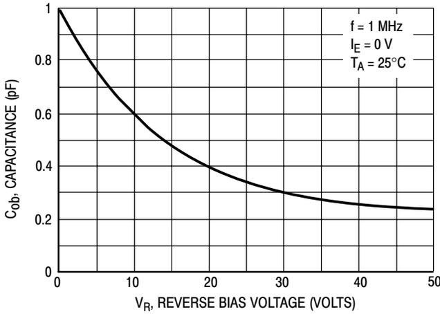
Figure 3. Output Capacitance
