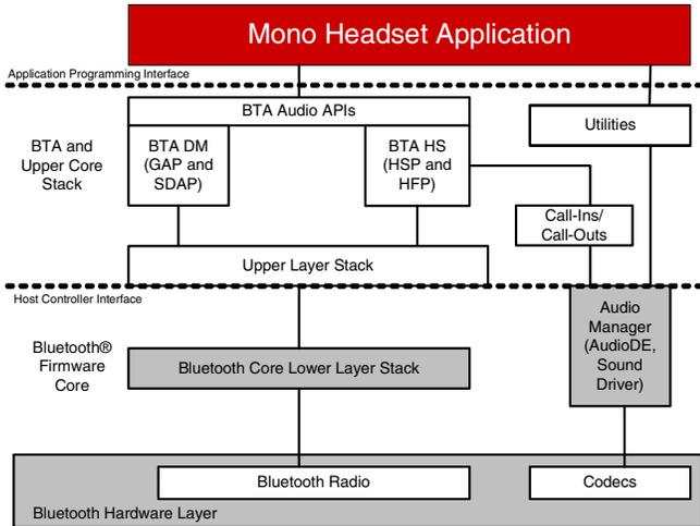
**Figure 1: BTA System Architecture for a Mono Headset**
