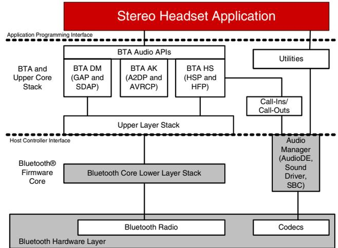
**Figure 2: BTA System Architecture for a Stereo Headset**
