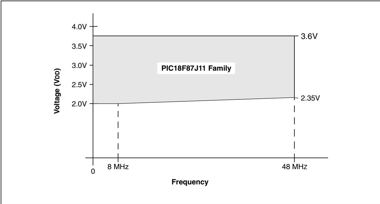
FIGURE 27-2: PIC18F87J11 FAMILY VOLTAGE-FREQUENCY GRAPH, REGULATOR DISABLED (INDUSTRIAL)<sup>(1)</sup>
