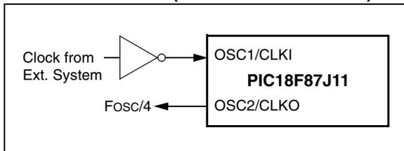
An external clock source may also be connected to the OSC1 pin in the HS mode, as shown in Figure 2-4. In this configuration, the divide-by-4 output on OSC2 is not available. Current consumption in this configuration will be somewhat higher than EC mode, as the internal oscillator's feedback circuitry will be enabled (in EC mode, the feedback circuit is disabled).
