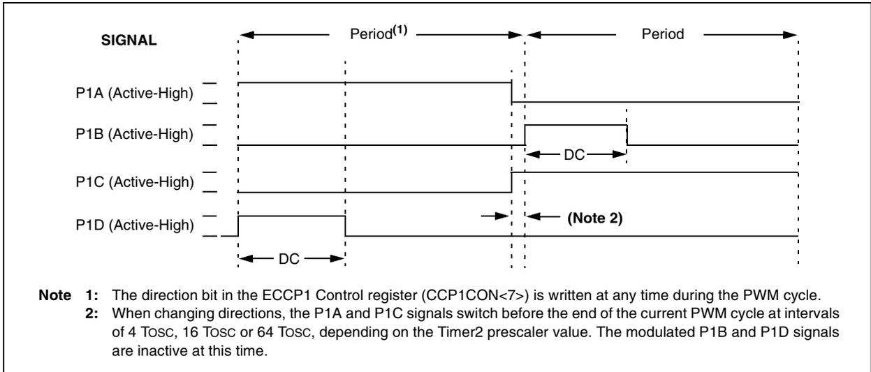
**FIGURE 18-9: PWM DIRECTION CHANGE AT NEAR 100% DUTY CYCLE**
