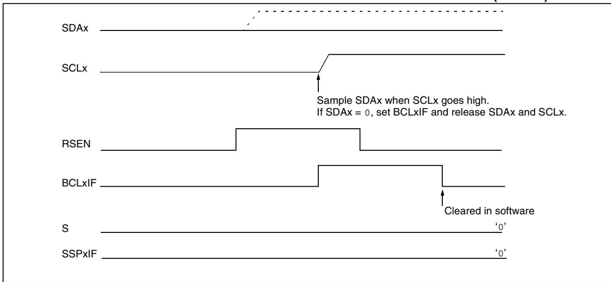
**FIGURE 19-32: BUS COLLISION DURING REPEATED START CONDITION (CASE 2)**
