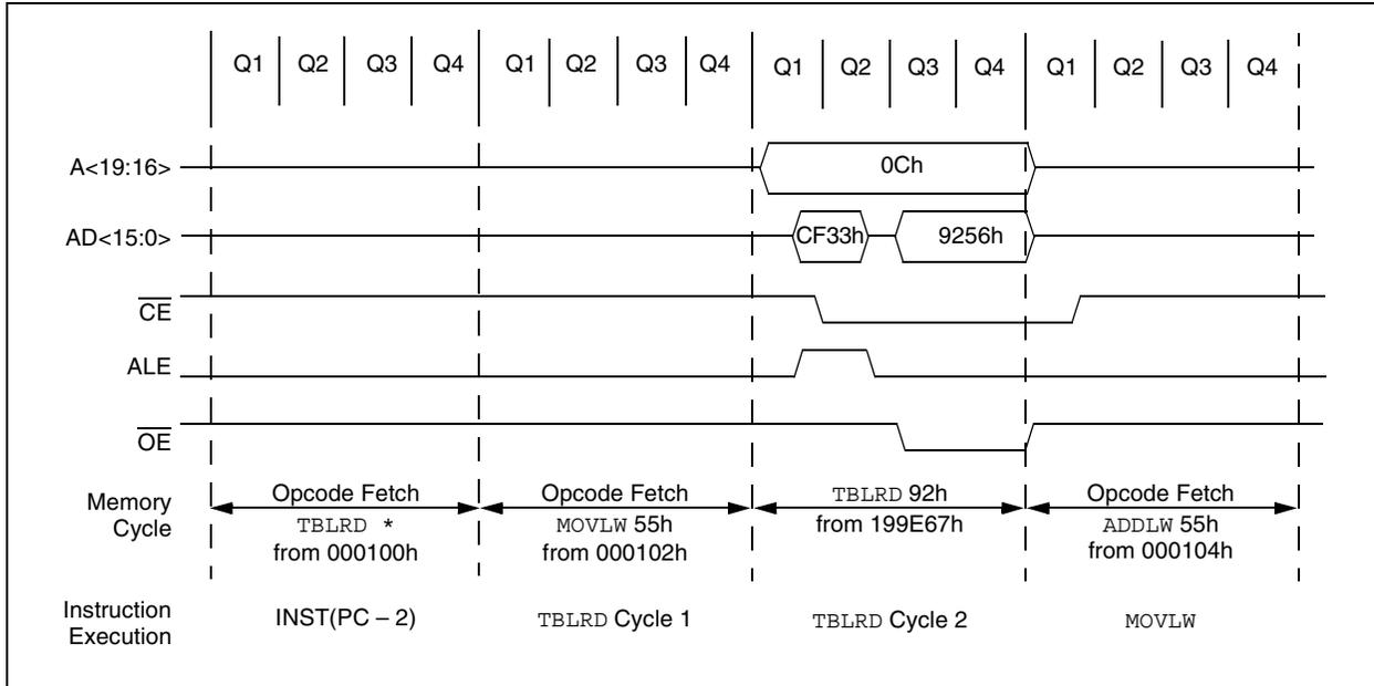
**FIGURE 7-5: EXTERNAL MEMORY BUS TIMING FOR SLEEP (EXTENDED MICROCONTROLLER MODE)**
