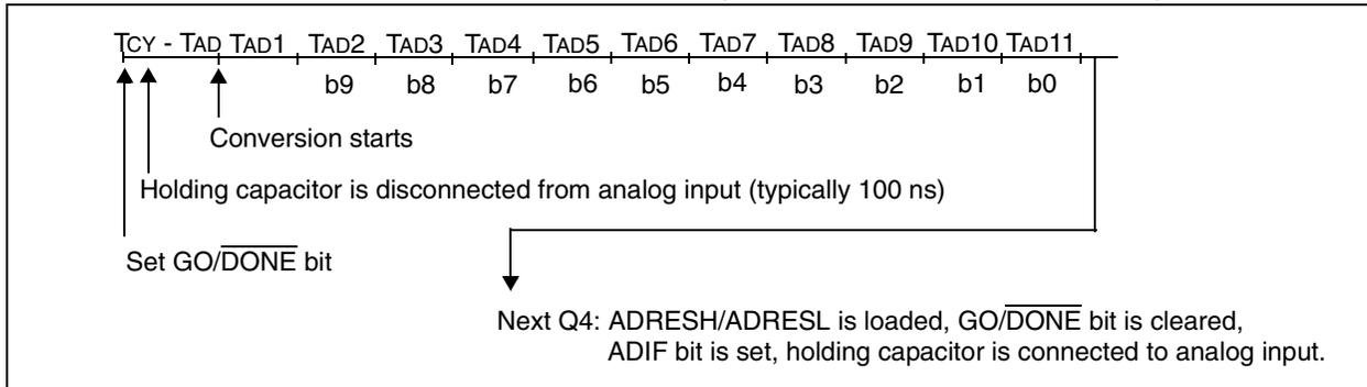
**FIGURE 21-4: A/D CONVERSION TAD CYCLES (ACQT2:ACQT0 = 010, TACQ = 4 TAD)**
