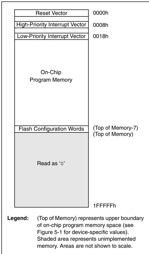
**Legend:** (Top of Memory) represents upper boundary of on-chip program memory space (see Figure 5-1 for device-specific values). Shaded area represents unimplemented memory. Areas are not shown to scale.
