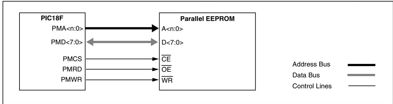
**FIGURE 11-31: PARALLEL EEPROM EXAMPLE (UP TO 15-BIT ADDRESS, 16-BIT DATA)**
