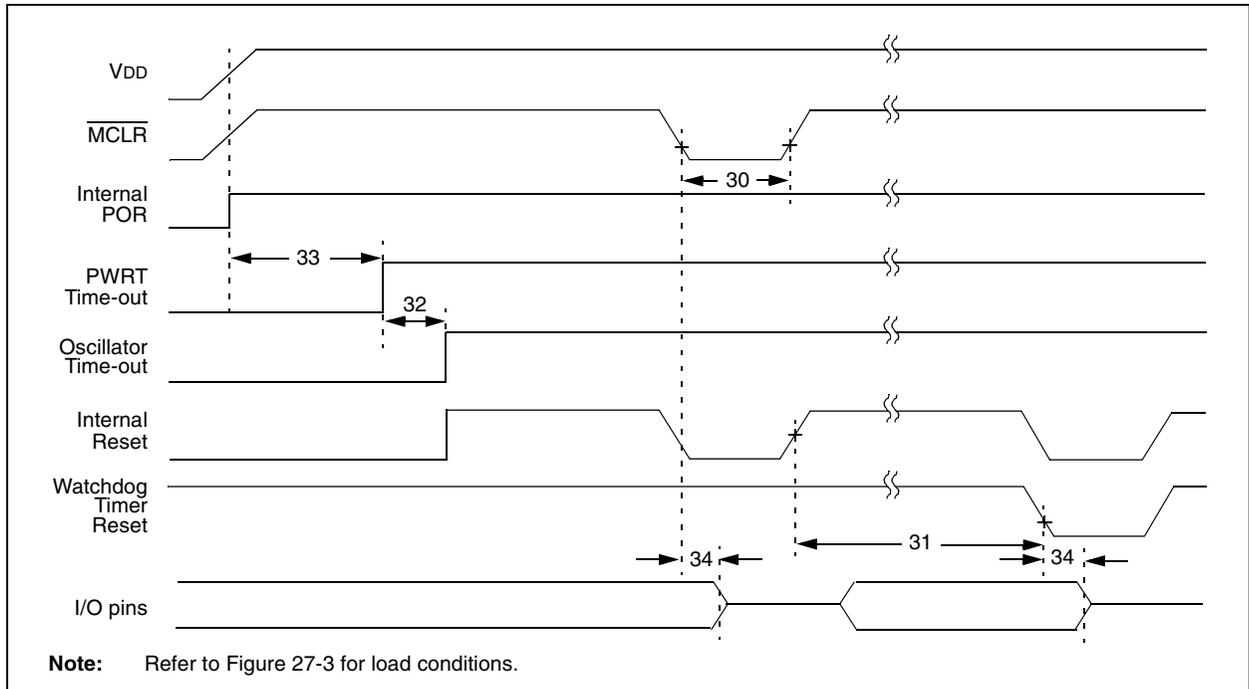
**TABLE 27-12: RESET, WATCHDOG TIMER, OSCILLATOR START-UP TIMER, POWER-UP TIMER AND BROWN-OUT RESET REQUIREMENTS**
