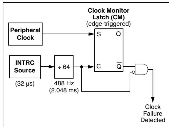
Clock failure is tested for on the falling edge of the sample clock. If a sample clock falling edge occurs while `CM` is still set, a clock failure has been detected (Figure 24-5). This causes the following:
