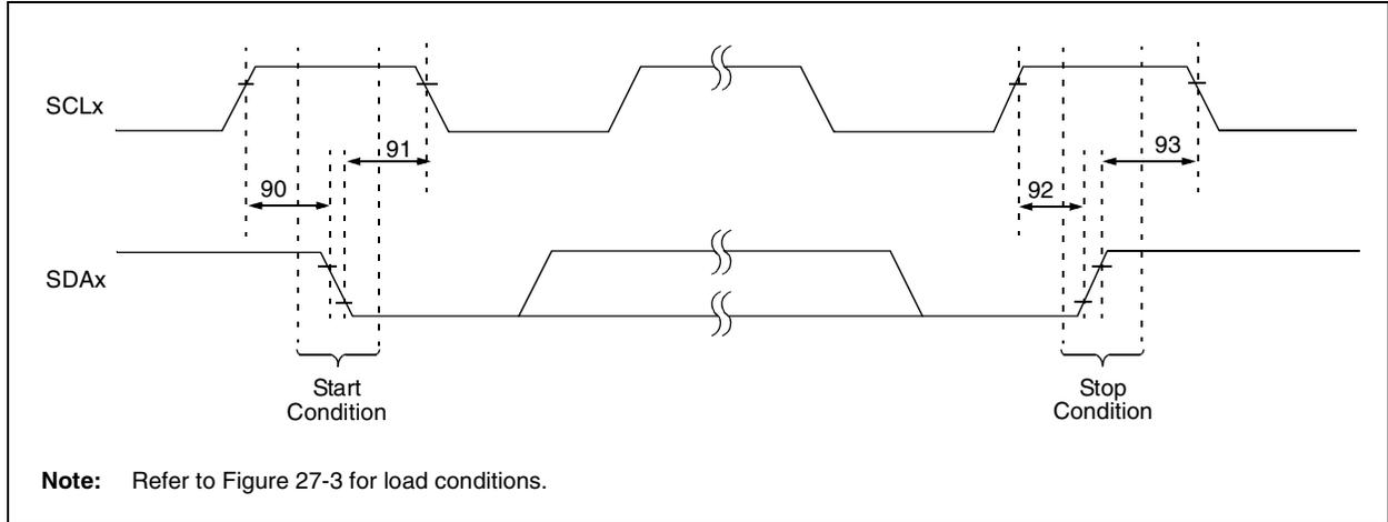
**TABLE 27-25: MSSP I<sup>2</sup>C™ BUS START/STOP BITS REQUIREMENTS**
