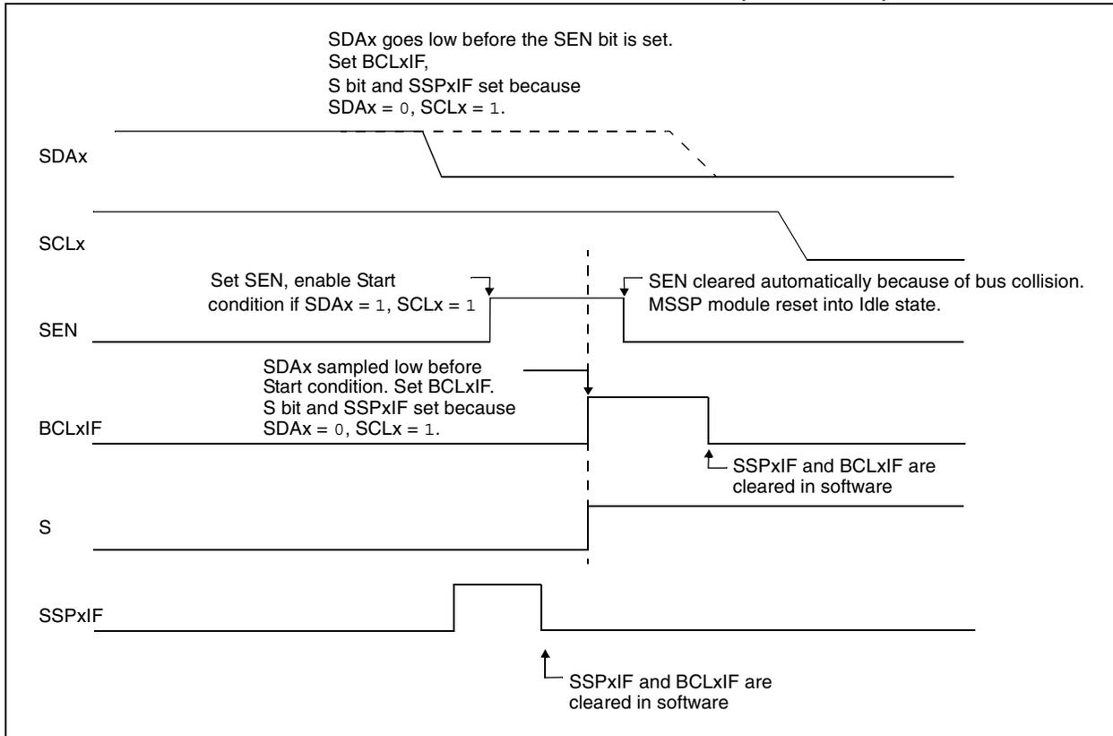
**FIGURE 19-29: BUS COLLISION DURING START CONDITION (SCLx = 0)**
