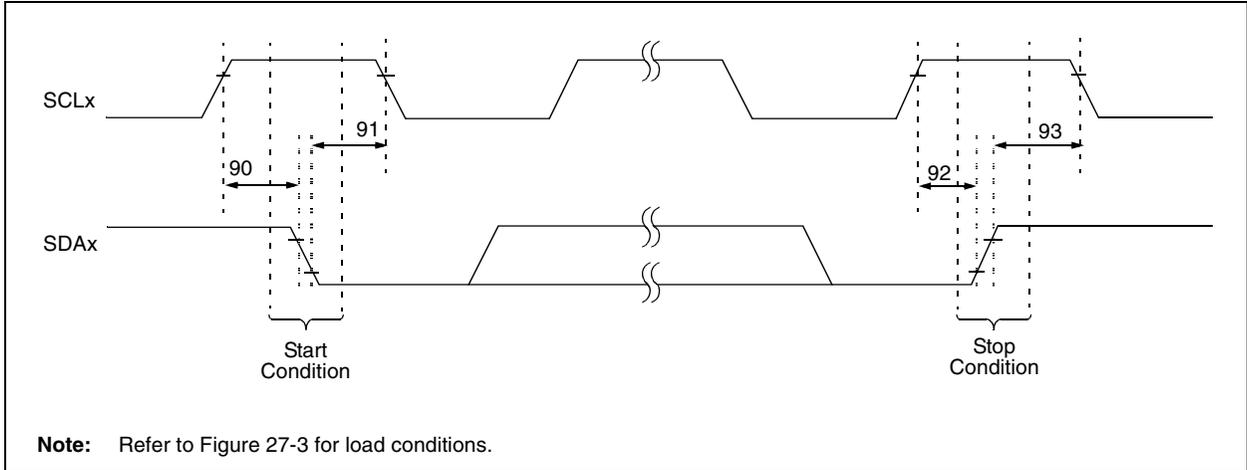
**TABLE 27-23: I<sup>2</sup>C™ BUS START/STOP BITS REQUIREMENTS (SLAVE MODE)**
