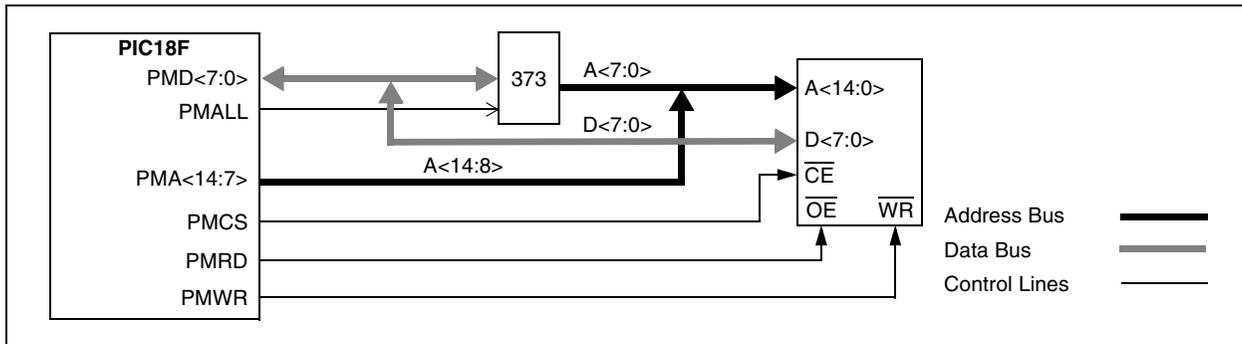
**FIGURE 11-29: EXAMPLE OF AN 8-BIT MULTIPLEXED ADDRESS AND DATA APPLICATION**
