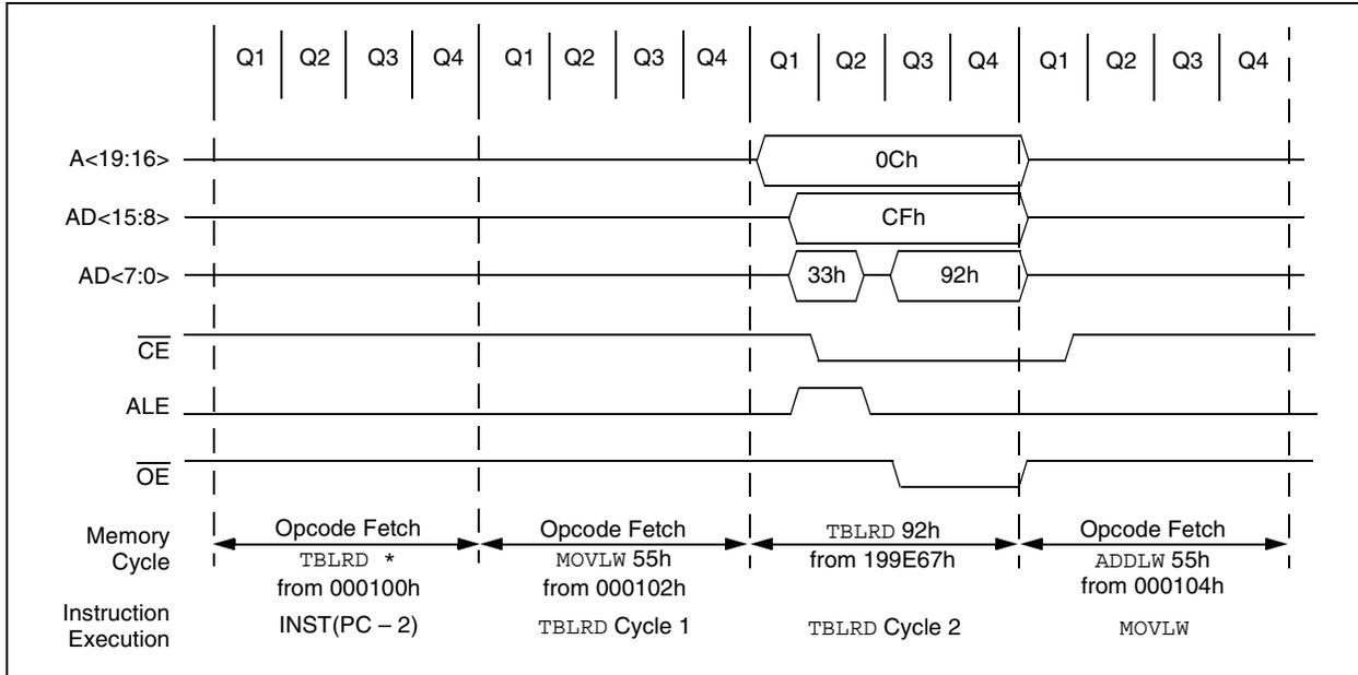
**FIGURE 7-8: EXTERNAL MEMORY BUS TIMING FOR SLEEP (EXTENDED MICROCONTROLLER MODE)**
