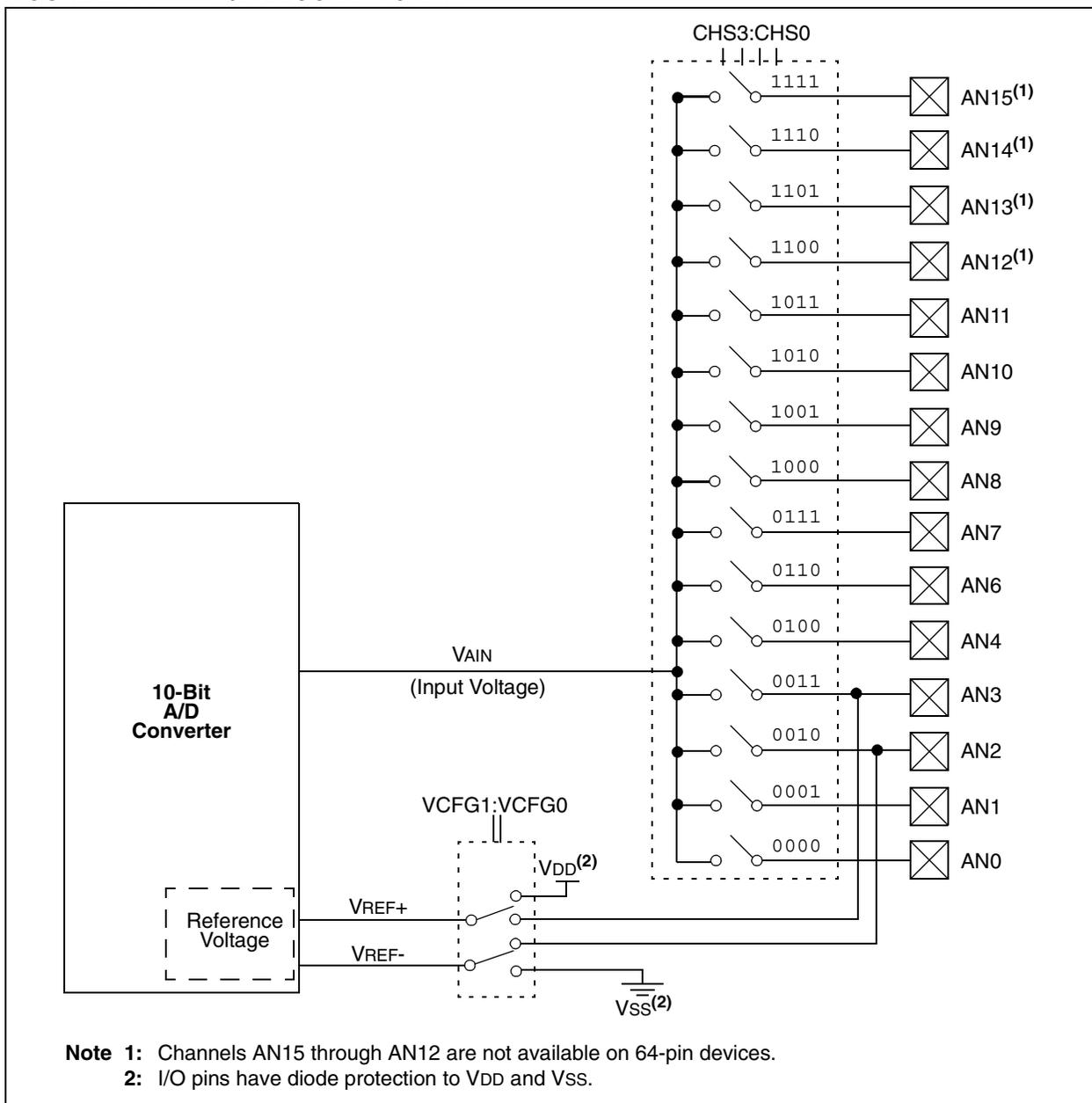
After the A/D module has been configured as desired, the selected channel must be acquired before the conversion is started. The analog input channels must have their corresponding TRIS bits selected as an input. To determine acquisition time, see **Section 21.1 “A/D Acquisition Requirements”**. After this acquisition time has elapsed, the A/D conversion can be started. An acquisition time can be programmed to occur between setting the GO/DONE bit and the actual start of the conversion.
