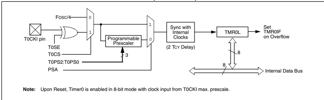
**FIGURE 12-2: TIMER0 BLOCK DIAGRAM (16-BIT MODE)**
