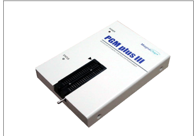
Figure 1-2 PGM-Plus (Single writer)
