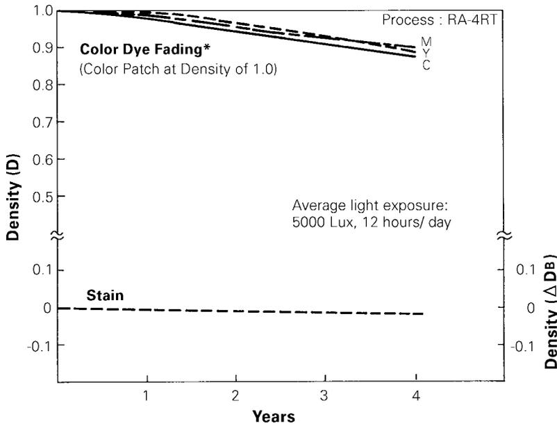
\* Time-lapse-induce white background staining (yellowing) is as important as dye image fading in affecting image quality. Therefore, dye image fading and yellowing data are also included.
