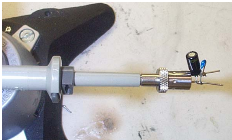
Figure 32 – Oscilloscope Probe with Probe Master 5125BA BNC Adapter (Modified for ripple measurement: wires for probe tip and ground with two decoupling capacitors connected in parallel).
