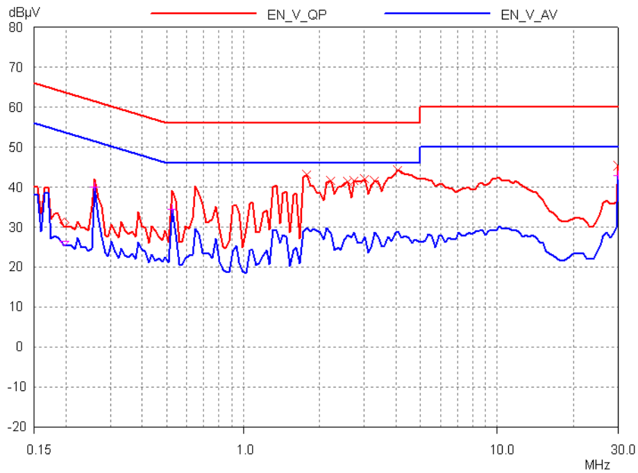
Figure 39 – Conducted EMI, Maximum Steady State Load, 230 VAC, 60 Hz, and EN55022 B Limits.
