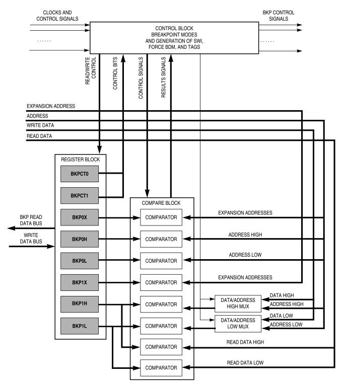
Figure 7-1. Breakpoint Block Diagram
