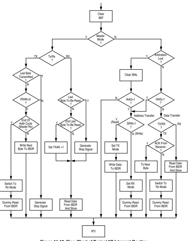
Figure 11-12. Flow-Chart of Typical IIC Interrupt Routine
