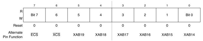
Figure 4-20. Port K Data Register (PORTK)
