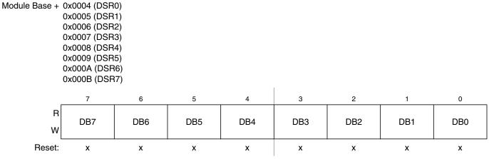
Figure 12-33. Data Segment Registers (DSR0–DSR7) — Extended Identifier Mapping
