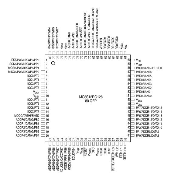
Figure 1-5. Pin assignments in 80 QFP for MC3S12RG128
