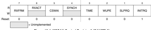
Figure 12-4. MSCAN Control Register 0 (CANCTL0)
