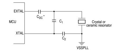
\* Due to the nature of a translated ground Colpitts oscillator a DC voltage bias is applied to the crystal
