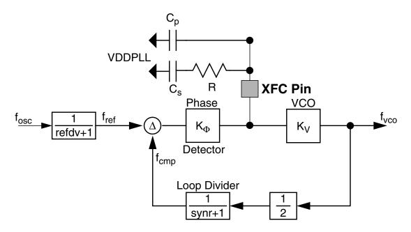
Figure A-3. Basic PLL functional diagram
