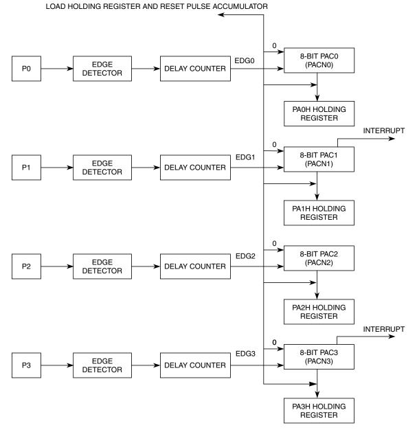
Figure 10-39. 8-Bit Pulse Accumulators Block Diagram
