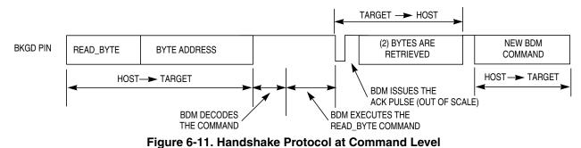
Differently from the normal bit transfer (where the host initiates the transmission), the serial interface ACK handshake pulse is initiated by the target MCU by issuing a falling edge in the BKGD pin. The hardware handshake protocol in Figure 6-10 specifies the timing when the BKGD pin is being driven, so the host
