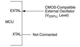
Figure 13-3. External Clock Connections (XCLKS = 1)
