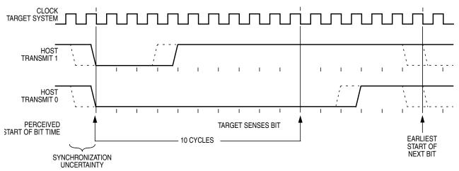
Figure 6-7. BDM Host-to-Target Serial Bit Timing
