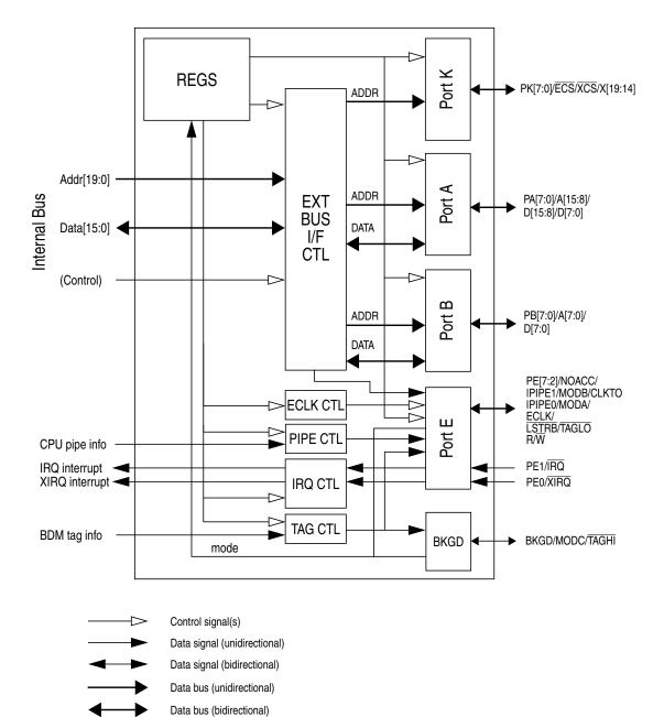
Figure 4-1. MEBI Block Diagram
