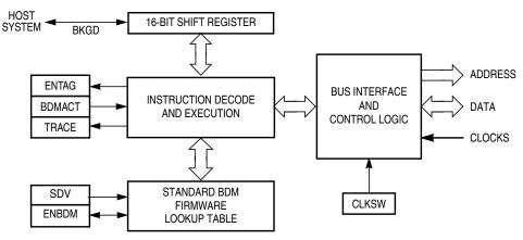
Figure 6-1. BDM Block Diagram
