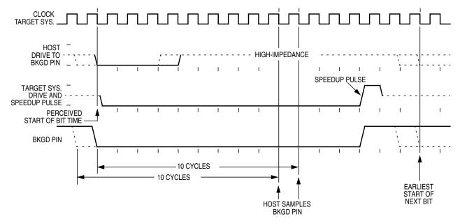
Figure 6-9. BDM Target-to-Host Serial Bit Timing (Logic 0)
