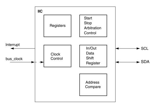
Figure 11-1. IIC Block Diagram
