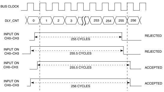
Figure 10-42. Channel Input Validity with Delay Counter Feature
