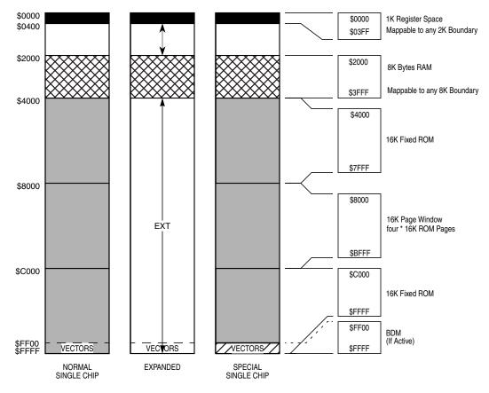
The figure shows a useful map, which is not the map out of reset. After reset the map is: \$0000 - \$03FF: Register Space \$0000 - \$1FFF: 8K RAM
