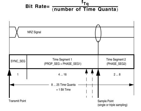
Figure 12-43. Segments within the Bit Time
