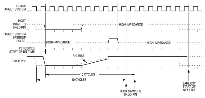
Figure 6-8. BDM Target-to-Host Serial Bit Timing (Logic 1)
