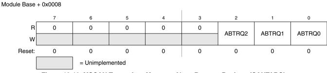
Figure 12-12. MSCAN Transmitter Message Abort Request Register (CANTARQ)
