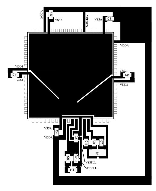
Figure C-2. Recommended PCB Layout for 80QFP Colpitts Oscillator
