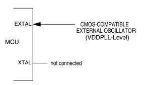
Figure 1-9. External Clock Connections (PE7=0)
