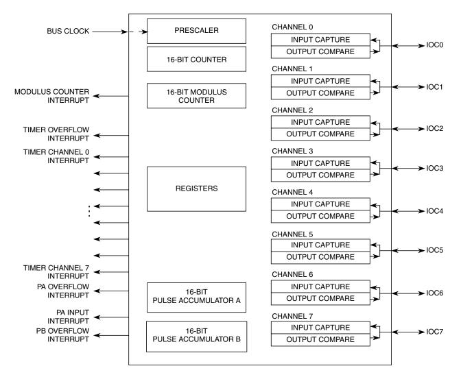
Figure 10-1. Timer Block Diagram
