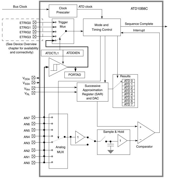
Figure 8-1. ATD Block Diagram
