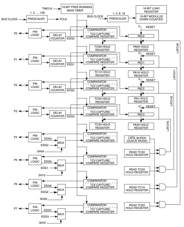
Figure 10-38. Detailed Timer Block Diagram in Queue Mode
