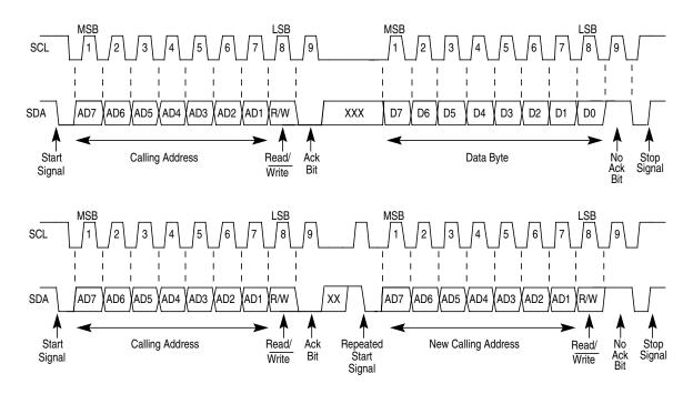
Figure 11-9. IIC-Bus Transmission Signals
