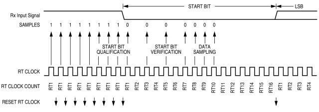
Figure 16-13. Receiver Data Sampling
