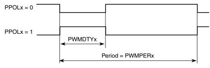
Figure 14-20. PWM Left Aligned Output Waveform
