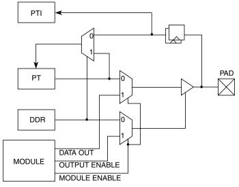
Figure 2-48. Illustration of I/O Pin Functionality
