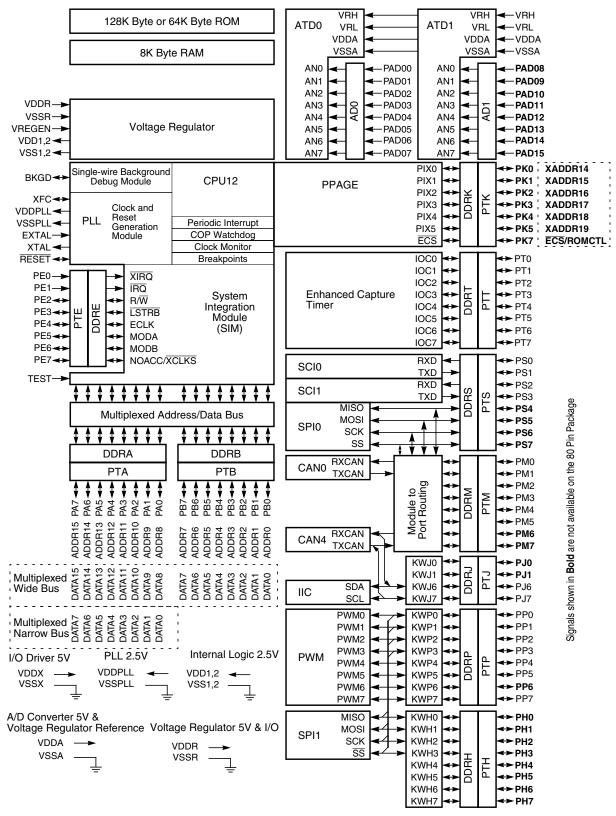
Figure 1-1. MC3S12RG128 Block Diagram
