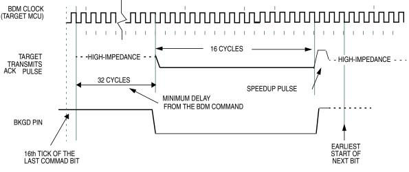
Figure 6-10. Target Acknowledge Pulse (ACK)
