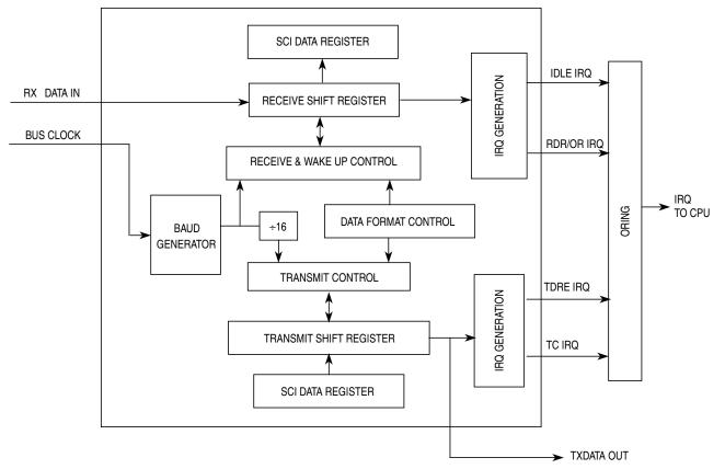
Figure 16-1. SCI Block Diagram
