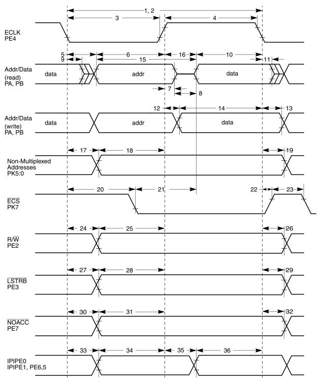
Figure A-10. General External Bus Timing
