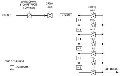
Figure 9-21. Clock Chain for COP
