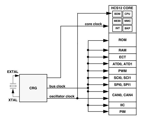
Figure 1-10. Clock Connections
