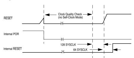
Figure 9-26. RESET Pin Tied to V<sub>DD</sub> (by a Pull-Up Resistor)
