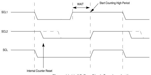
Figure 11-11. IIC-Bus Clock Synchronization
