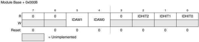
Figure 12-15. MSCAN Identifier Acceptance Control Register (CANIDAC)
