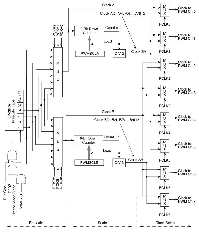
Figure 14-18. PWM Clock Select Block Diagram
