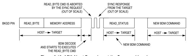
Figure 6-12. ACK Abort Procedure at the Command Level
