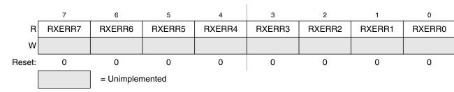
Figure 12-17. MSCAN Receive Error Counter (CANRXERR)
