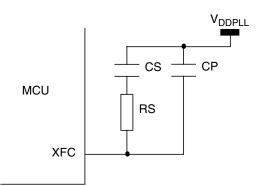
Figure 9-2. PLL Loop Filter Connections
