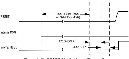
Figure 9-27. RESET Pin Held Low Externally
