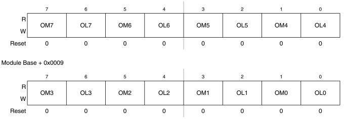
Figure 10-10. Timer Control Register 1/Timer Control Register 2 (TCTL1/TCTL2))
