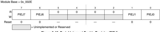
Figure 2-46. Port J Interrupt Enable Register (PIEJ)
