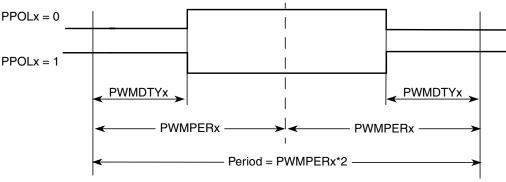
Figure 14-22. PWM Center Aligned Output Waveform
