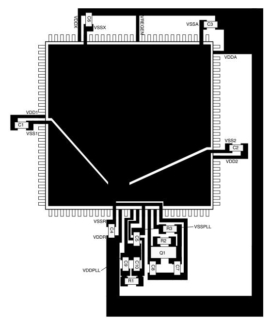
Figure C-3. Recommended PCB Layout for 112LQFP Pierce Oscillator
