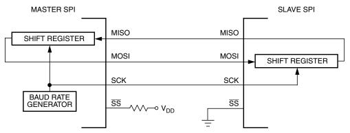
Figure 17-8. Master/Slave Transfer Block Diagram
