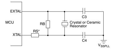
\* Rs can be zero (shorted) when used with higher frequency crystals. Refer to manufacturer's data.
