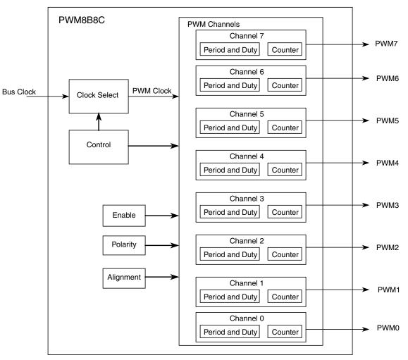
Figure 14-1. PWM Block Diagram
