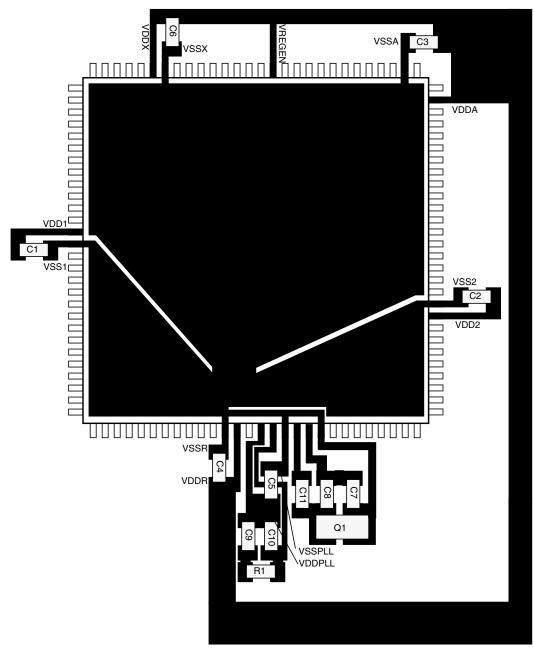
Figure C-1. Recommended PCB Layout for 112LQFP Colpitts Oscillator
