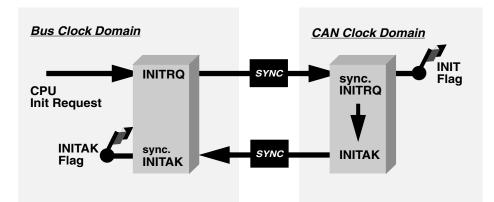
Figure 12-46. Initialization Request/Acknowledge Cycle
