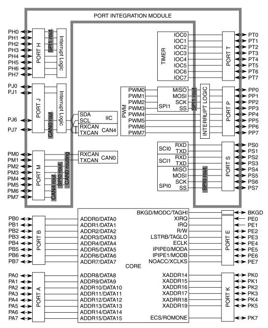
Figure 2-1. PIM3RG128 Block Diagram
