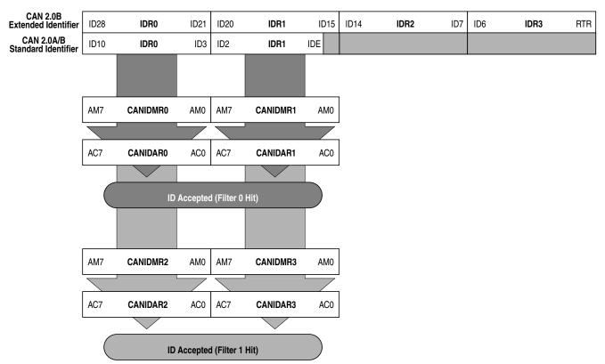
Figure 12-40. 16-bit Maskable Identifier Acceptance Filters
