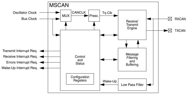
Figure 12-1. MSCAN Block Diagram
