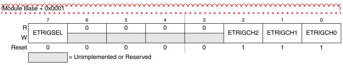
Figure 8-4. ATD Control Register 1 (ATDCTL1)
