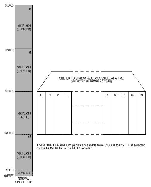
Figure 3-11. Memory Paging Example: 1M Byte On-Chip FLASH/ROM, 64K Allocation
