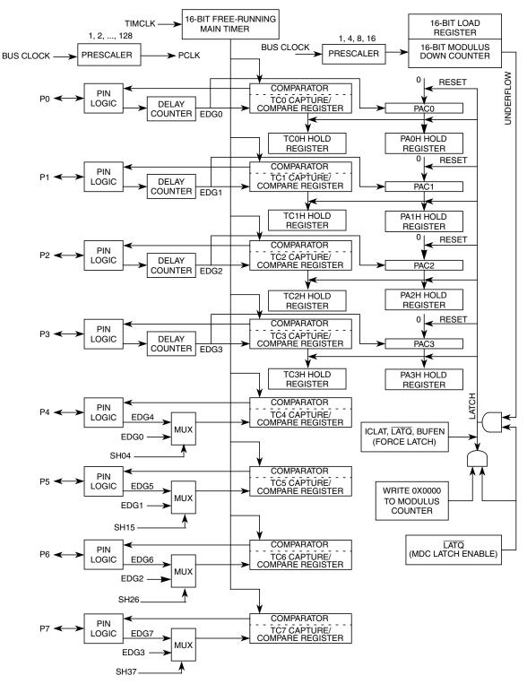
Figure 10-37. Detailed Timer Block Diagram in Latch Mode
