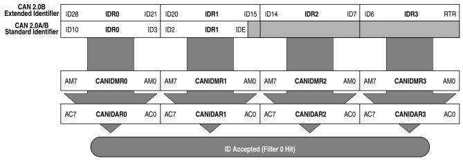
Figure 12-39. 32-bit Maskable Identifier Acceptance Filter
