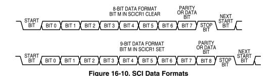
Each data character is contained in a frame that includes a start bit, eight or nine data bits, and a stop bit. Clearing the M bit in SCI control register 1 configures the SCI for 8-bit data characters. A frame with eight data bits has a total of 10 bits. Setting the M bit configures the SCI for nine-bit data characters. A frame with nine data bits has a total of 11 bits
