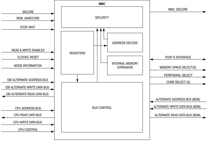
Figure 3-1. MMC Block Diagram
