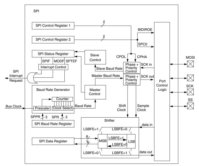
Figure 17-1. SPI Block Diagram
