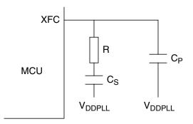
Figure 1-6. PLL Loop Filter Connections
