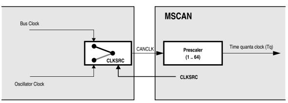
Figure 12-42. MSCAN Clocking Scheme
