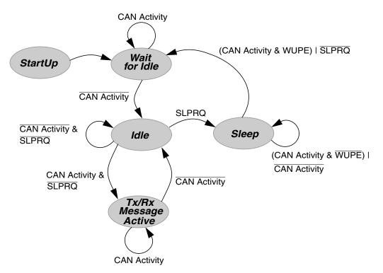
Figure 12-45. Simplified State Transitions for Entering/Leaving Sleep Mode
