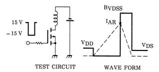
$$\begin{array}{l} T_{ch} = 25^{\circ}C \ (Initial) \\ Peak \ I_{AR} = -3.5 \ A, \ R_G = 25 \ \Omega \\ V_{DD} = -24 \ V, \ L = 1.48 \ mH \end{array} \\ E_{AS} = \frac{1}{2} \cdot L \cdot I^2 \cdot ( \ \frac{B_{VDSS}}{B_{VDSS} - V_{DD}}) \\ \end{array} \label{eq:continuous}$$
