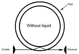
If the diameter of the pipe is close to 6 mm, some of the emitted light may reach the receiver because the angle of refraction is small. This may result in false readings. In such cases, set the sensitivity selector to Low and check that the EE-SPX613 reads correctly for pipes with and without liquid.
