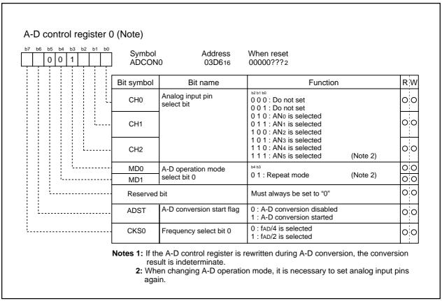
Figure 2.12.8 A-D conversion register 0 in repeat mode
