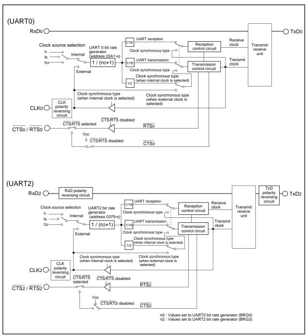
Figure 2.11.1 Block diagram of UARTi (i = 0 and 2)
