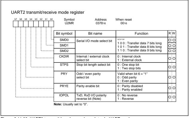
Figure 2.11.22 UART2 transmit/receive mode register in UART mode
