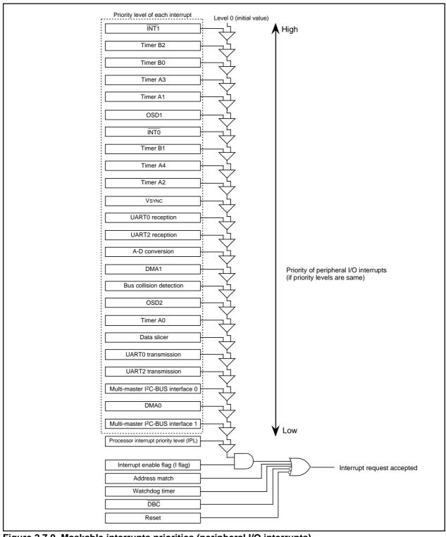
Figure 2.7.9 Maskable interrupts priorities (peripheral I/O interrupts)
