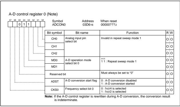
Figure 2.12.14 A-D control register 0 in repeat sweep mode 1
