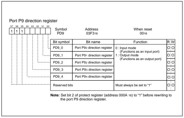
Figure 2.17.9 Port P9 direction register
