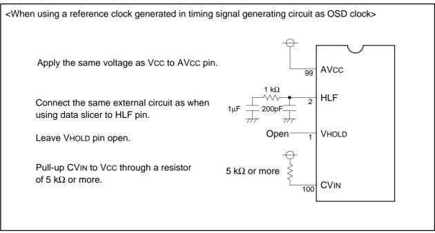
Figure 2.14.3 Termination of data slicer input/output pins when timing signal generating circuit is in ON state
