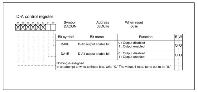
Figure 2.13.2 D-A control register
