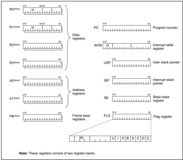
Figure 2.2.1 Central processing unit register
