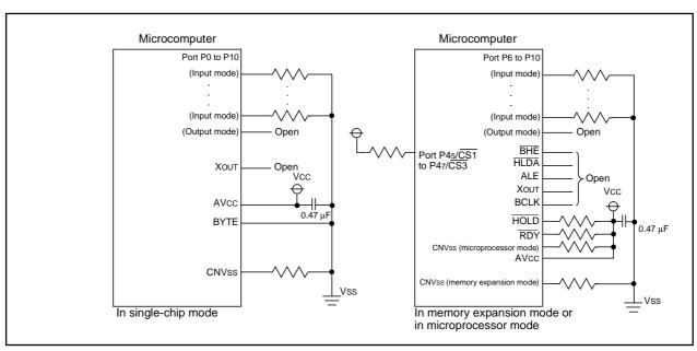
Figure 2.17.18 Example connection of unused pins
