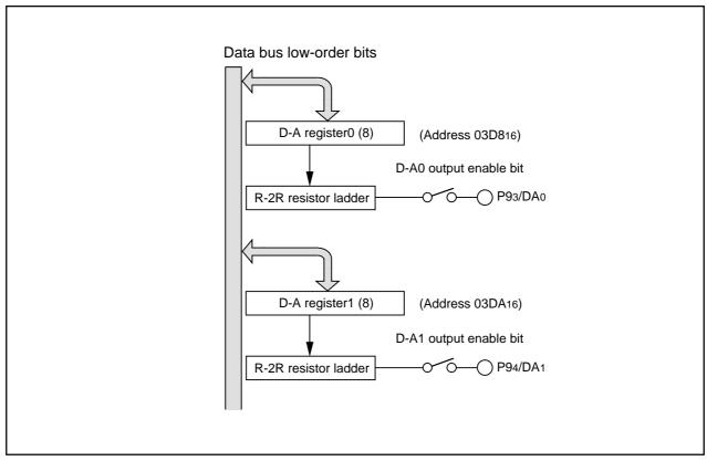
Figure 2.13.1 Block diagram of D-A converter
