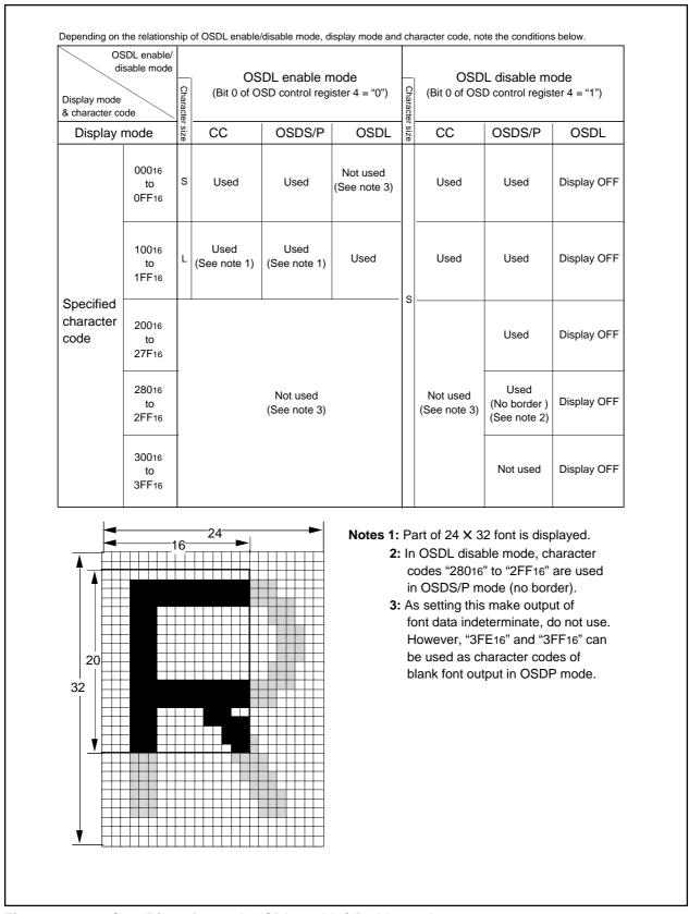
Figure 2.16.22 Conditions for each OSDL enable/disable mode
