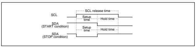
Fig. 2.11.44 START condition/STOP condition detect timing diagram
