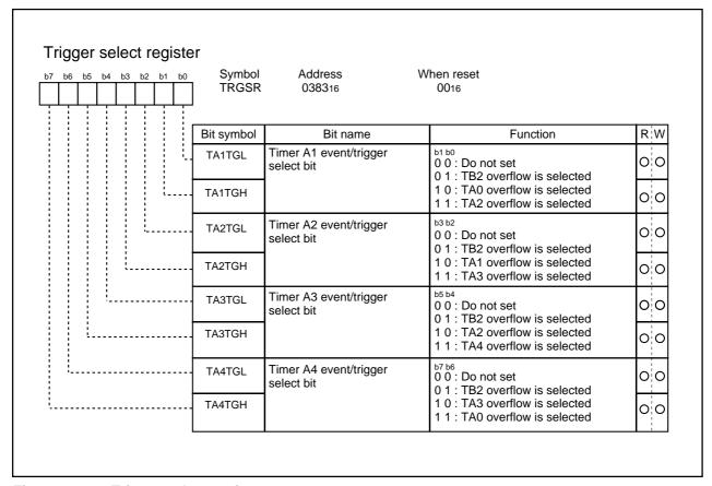
Figure 2.10.9 Trigger select register
