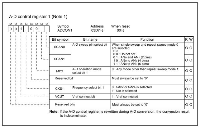
Figure 2.12.11 A-D control register 1 in single sweep mode
