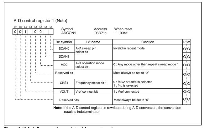
Figure 2.12.9 A-D conversion register 1 in repeat mode
