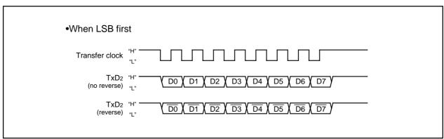
Figure 2.11.20 Serial data logic switch timing
