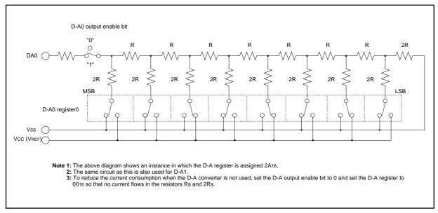
Figure 2.13.4 D-A converter equivalent circuit
