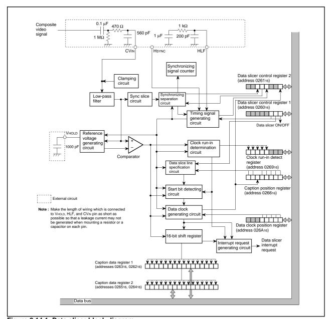
Figure 2.14.1 Data slicer block diagram
