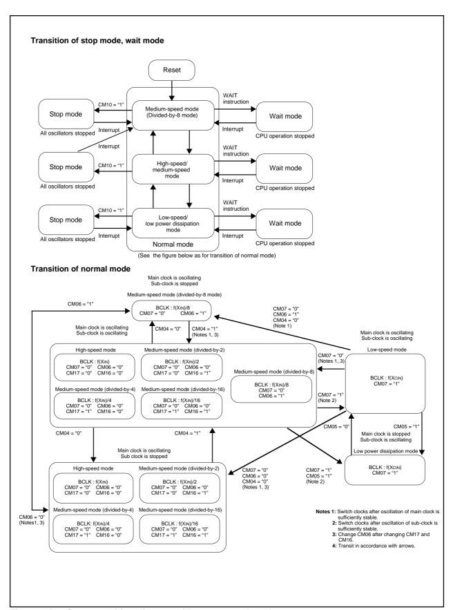
Figure 2.5.7 State transition diagram of Power control mode
