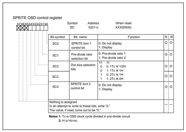
Figure 2.16.42 SPRITE OSD control register
