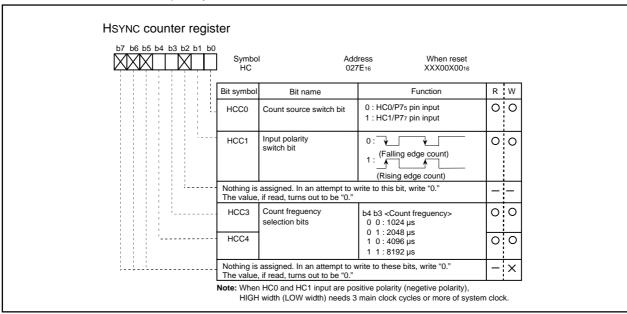
Figure 2.15.1 HSYNC counter register
