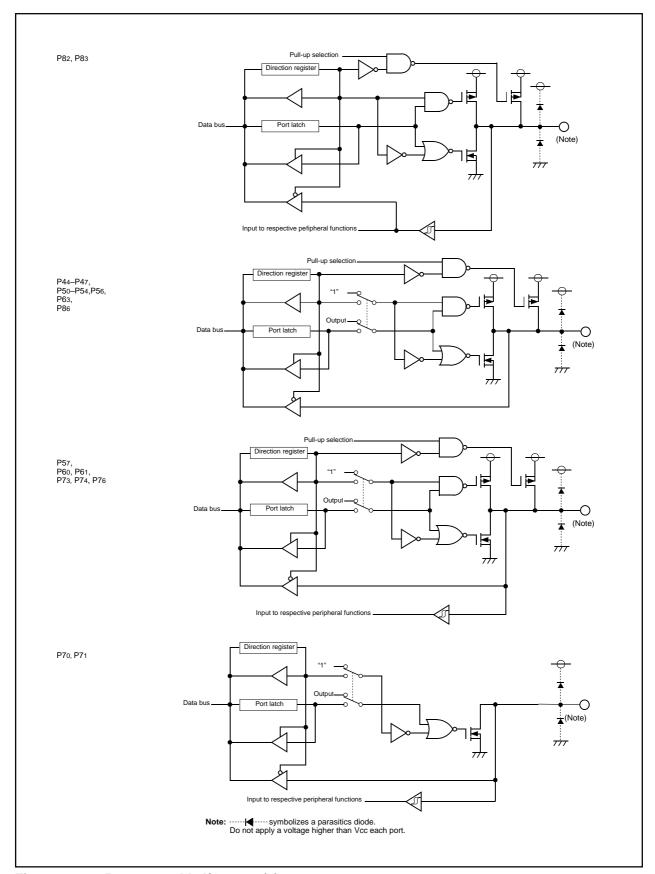
Figure 2.17.2 Programmable I/O ports (3)
