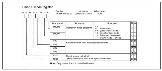
Figure 2.10.4 Timer Ai mode register (i = 0 to 4)
