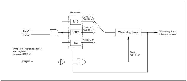
Figure 2.8.1 Block diagram of watchdog timer
