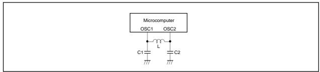
Figure 2.5.3 OSD clock connection example
