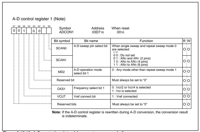
Figure 2.12.13 A-D control register 1 in repeat sweep mode 0
