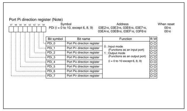
Figure 2.17.6 Port Pi direction register (i = 0 to 10, except 6, 8, 9)
