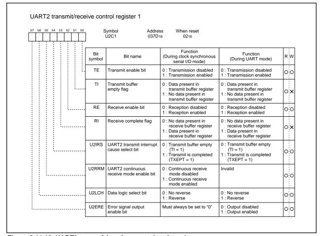
Figure 2.11.12 UART2 transmit/receive control register 1
