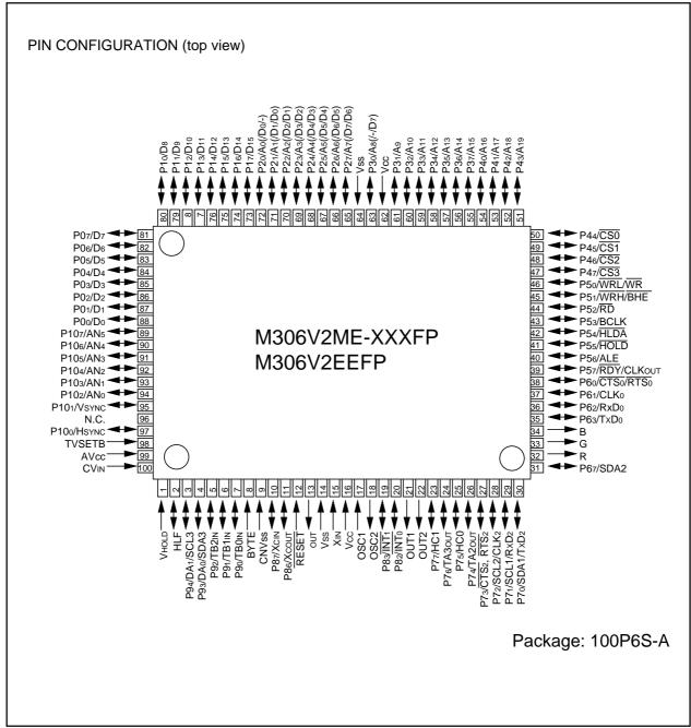
Figure 1.3.1 Pin configuration (top view)
