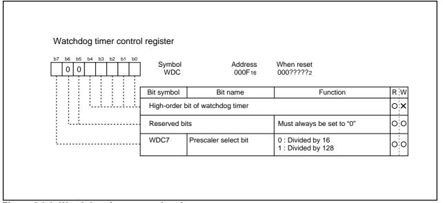
Figure 2.8.2 Watchdog timer control register
