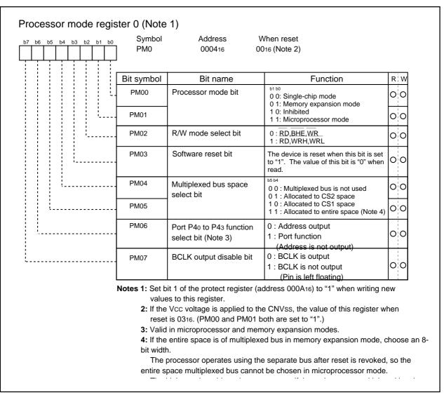
Figure 2.4.1 Processor mode register 0
