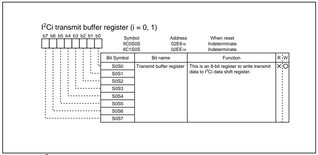
Fig. 2.11.36  $I^2$ Ci transmit buffer register (i = 0, 1)
