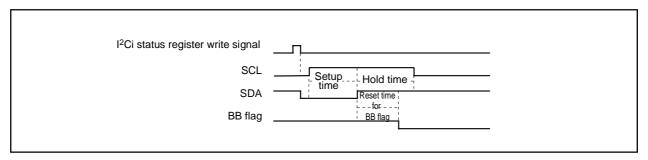
Fig. 2.11.43 STOP condition generation timing diagram
