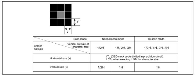
Figure 2.16.35 Horizontal and vertical size of border
