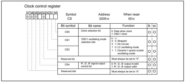
Figure 2.16.15 Clock control register
