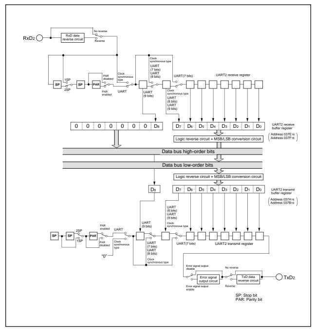
Figure 2.11.3 Block diagram of UART2 transmit/receive unit
