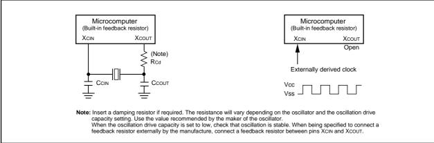
Figure 2.5.2 Examples of sub-clock
