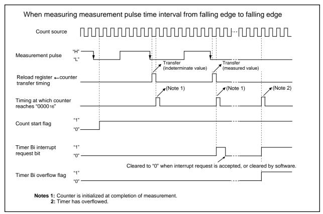
Figure 2.10.24 Operation timing when measuring a pulse period
