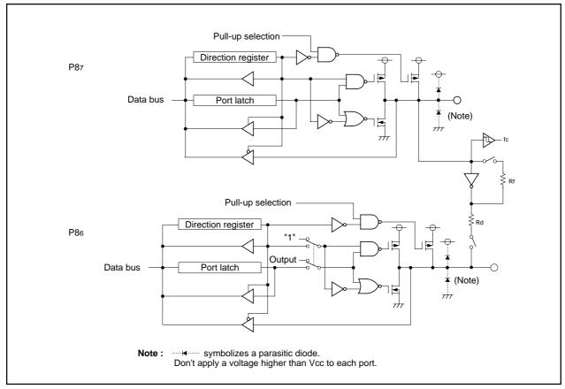
Figure 2.17.4 Programmable I/O ports (4)
