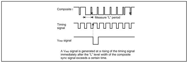
Figure 2.14.6 Vsep generating timing (method 2)
