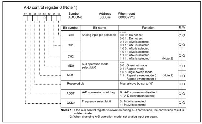
Figure 2.12.2 A-D control register 0
