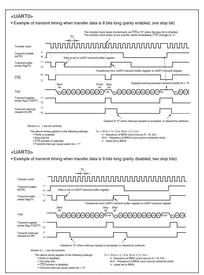
Figure 2.11.23 Typical transmit/receive timings in UART mode
