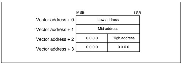
Figure 2.7.2 Format for specifying interrupt vector addresses
