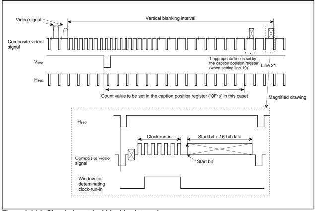
Figure 2.14.8 Signals in vertical blanking interval
