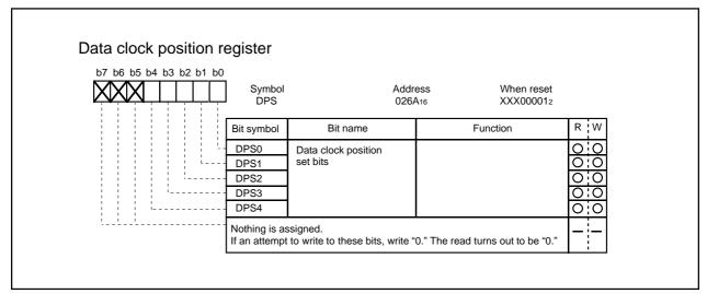
Figure 2.14.11 Data clock position register
