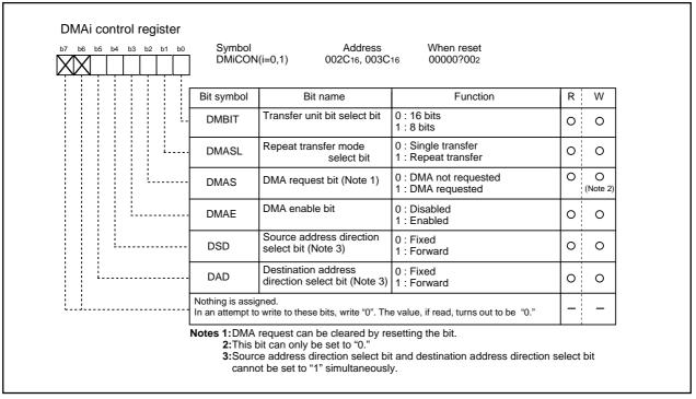
Figure 2.9.4 DMAi control register (i = 0, 1)
