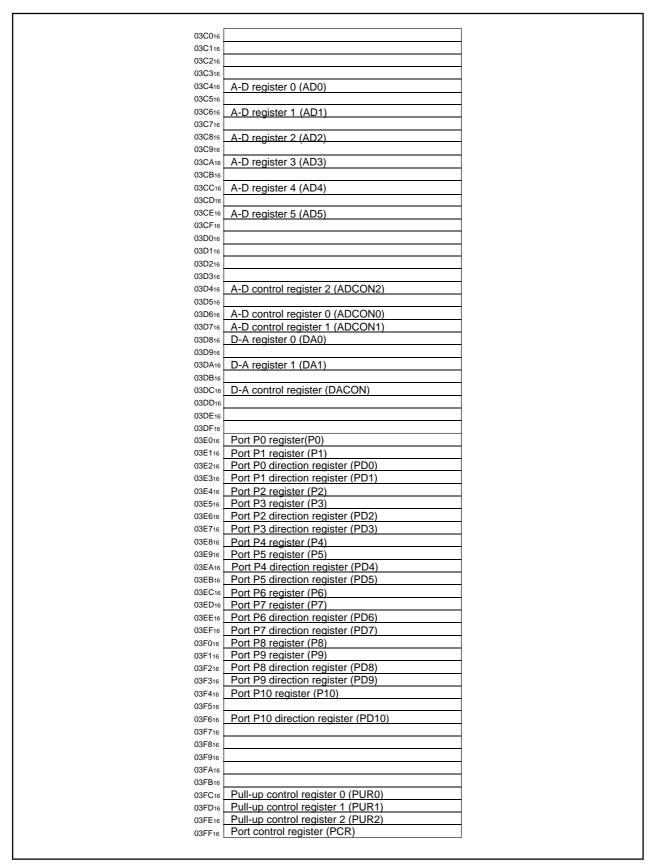
Figure 2.1.5 Location of peripheral unit control registers (4)
