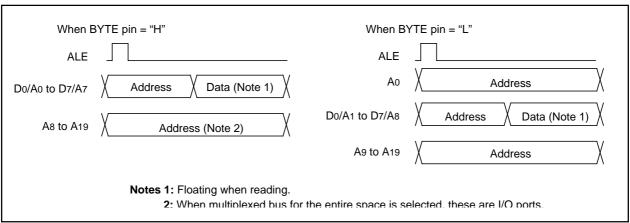
Figure 2.4.5 ALE signal and address/data bus
