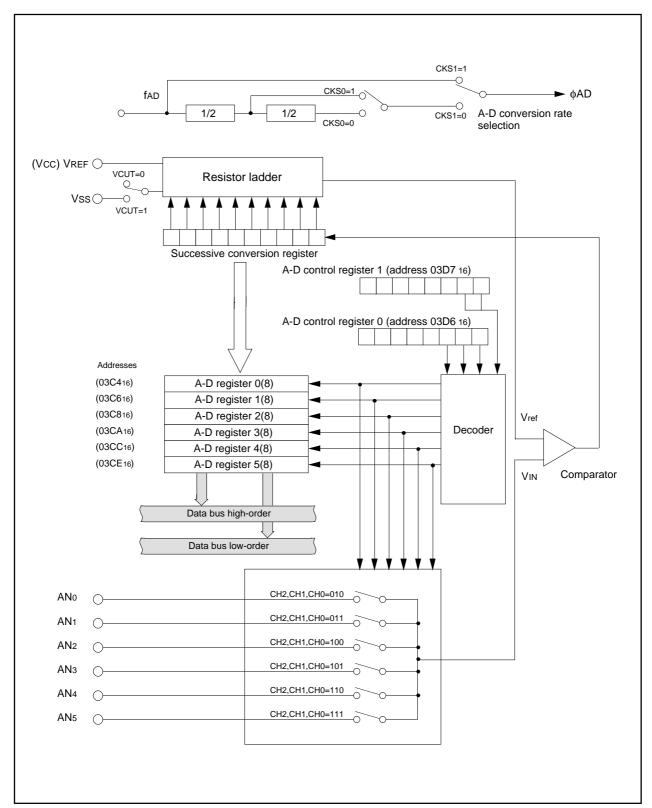
Figure 2.12.1 Block diagram of A-D converter
