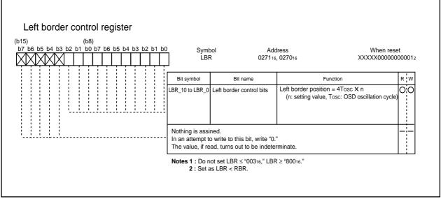
Figure 2.16.49 Left border control register
