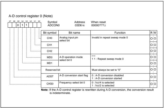
Figure 2.12.12 A-D control register 0 in repeat sweep mode 0
