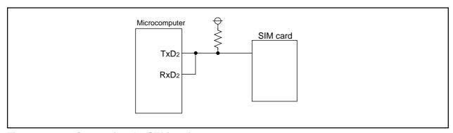
Figure 2.11.30 Connecting the SIM interface
