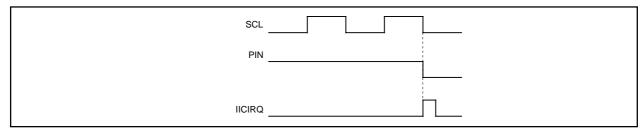
Fig. 2.11.41 Interrupt request signal generation timing
