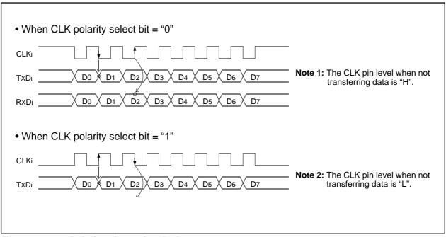
Figure 2.11.18 Polarity of transfer clock
