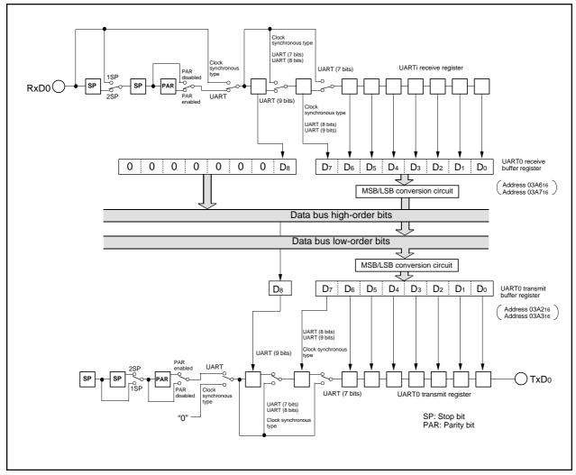
Figure 2.11.2 Block diagram of UART0 transmit/receive unit
