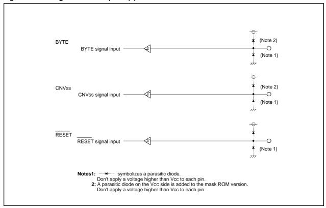
Figure 2.17.5 I/O pins
