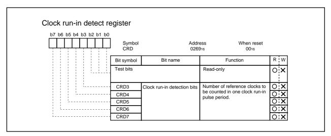
Figure 2.14.10 Clock run-in detect register
