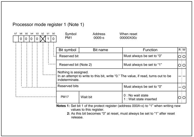
Figure 2.4.2 Processor mode register 1
