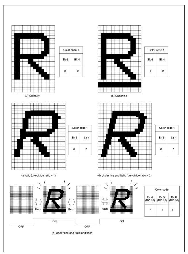
Figure 2.16.32 Example of attribute display (in CC mode)
