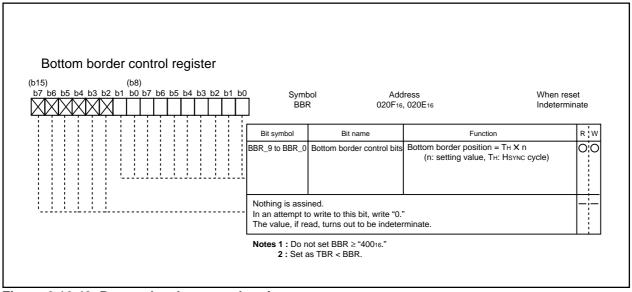
Figure 2.16.48 Bottom border control register
