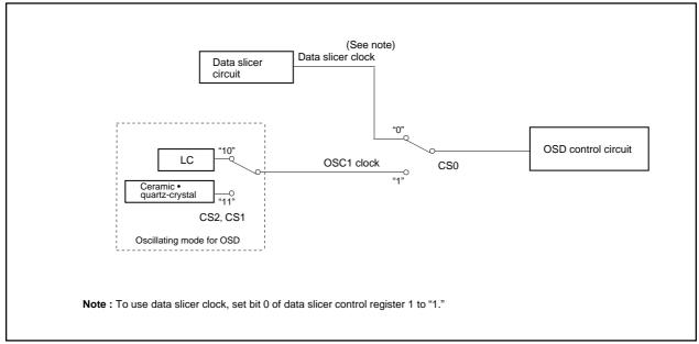
Figure 2.16.16 Block Diagram of OSD selection circuit
