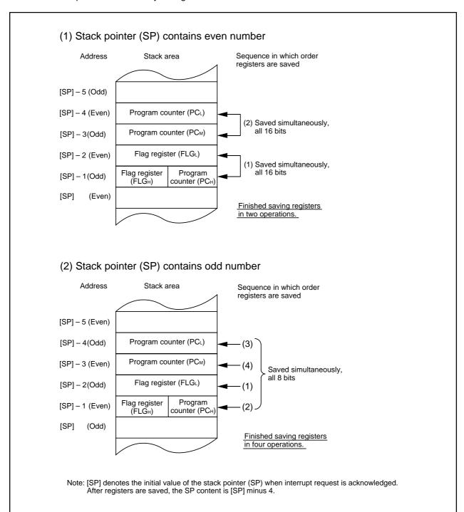
Figure 2.7.7 Operation of saving registers
