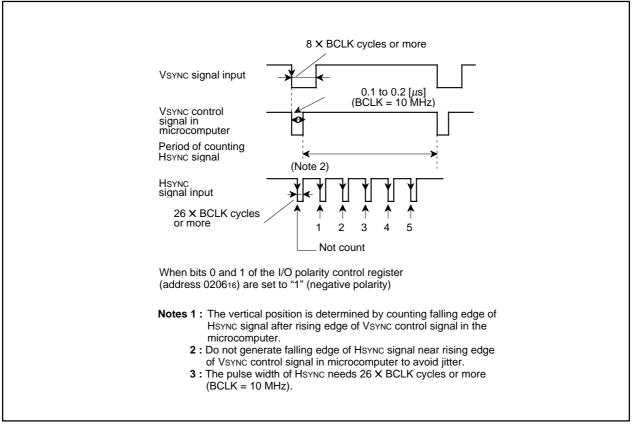
Figure 2.16.9 Supplement explanation for display position
