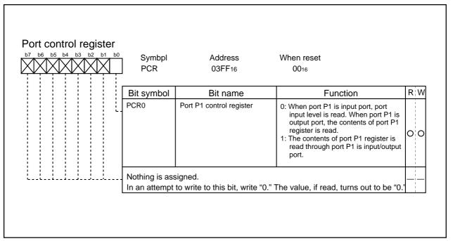
Figure 2.17.14 Port control register
