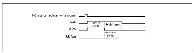
Fig. 2.11.42 START condition generation timing diagram
