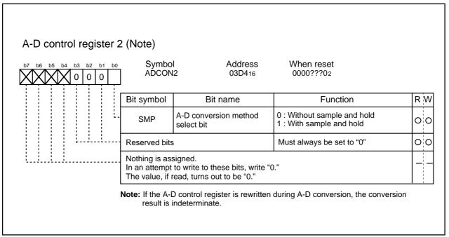
Figure 2.12.4 A-D control register 2
