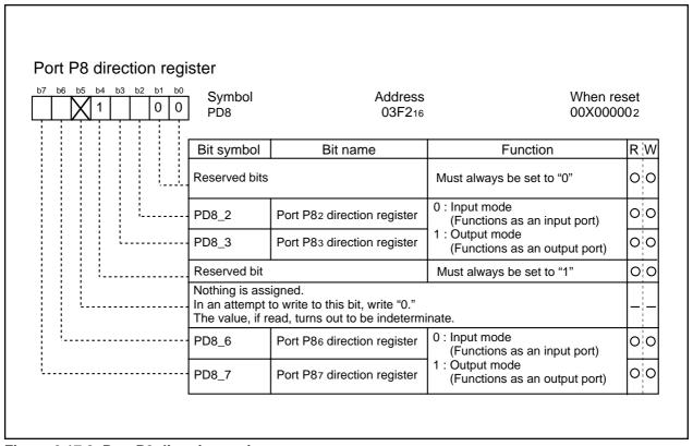
Figure 2.17.8 Port P8 direction register
