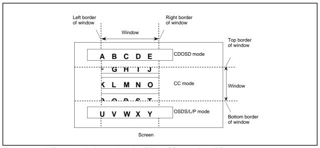
Figure 2.16.45 Example of window function (When CC mode is valid)
