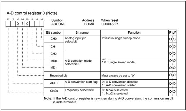
Figure 2.12.10 A-D control register 0 in single sweep mode
