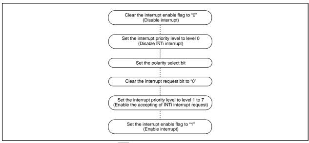
Figure 2.7.14 Switching condition of INT interrupt request
