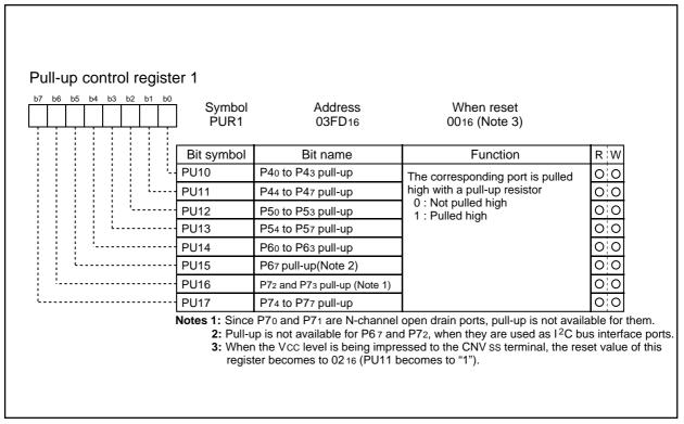
Figure 2.17.16 Pull-up control register 1
