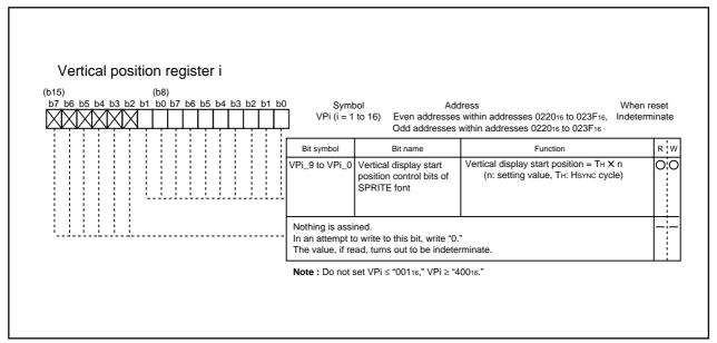
Figure 2.16.10 Vertical position register i (i = 1 to 16)
