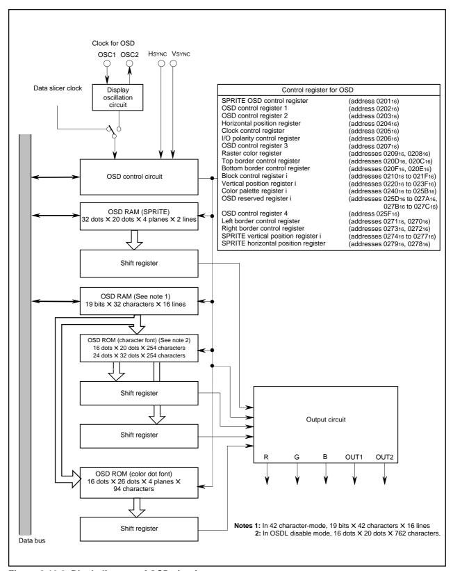
Figure 2.16.2 Block diagram of OSD circuit
