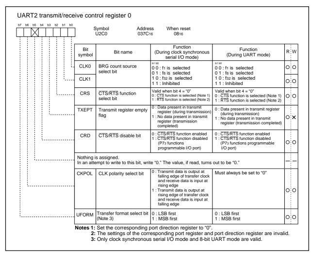
Figure 2.11.10 UART2 transmit/receive control register 0
