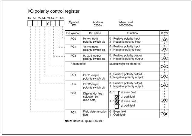
Figure 2.16.17 I/O polarity control register
