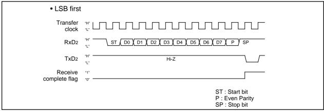
Figure 2.11.28 Output timing of the parity error signal
