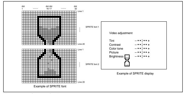
Figure 2.16.41 SPRITE OSD display example
