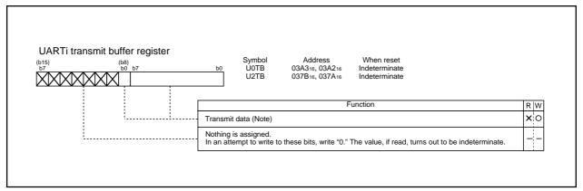
Figure 2.11.4 UARTi transmit buffer register (i = 0 and 2)
