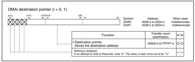
Figure 2.9.6 DMAi destination pointer (i = 0, 1)
