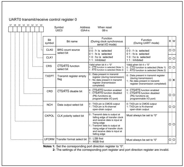
Figure 2.11.9 UART0 transmit/receive control register 0
