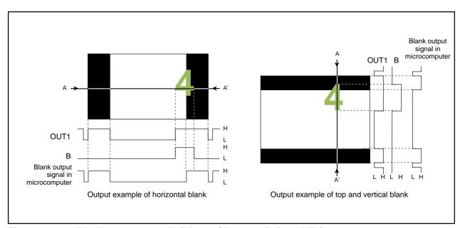
Figure 2.16.46 Blank output example (when OSD output is B + OUT1)
