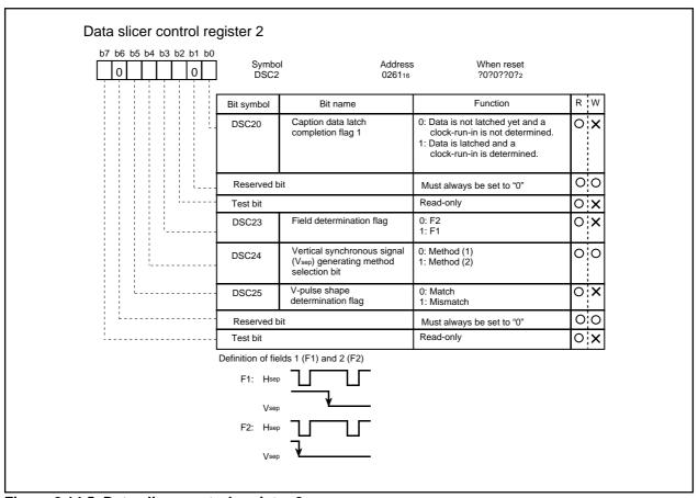
Figure 2.14.5 Data slicer control register 2
