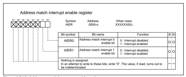
Figure 2.7.12 Address match interrupt enable register
