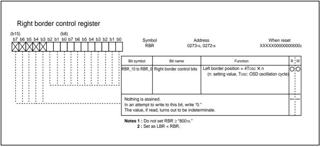
Figure 2.16.50 Right border control register
