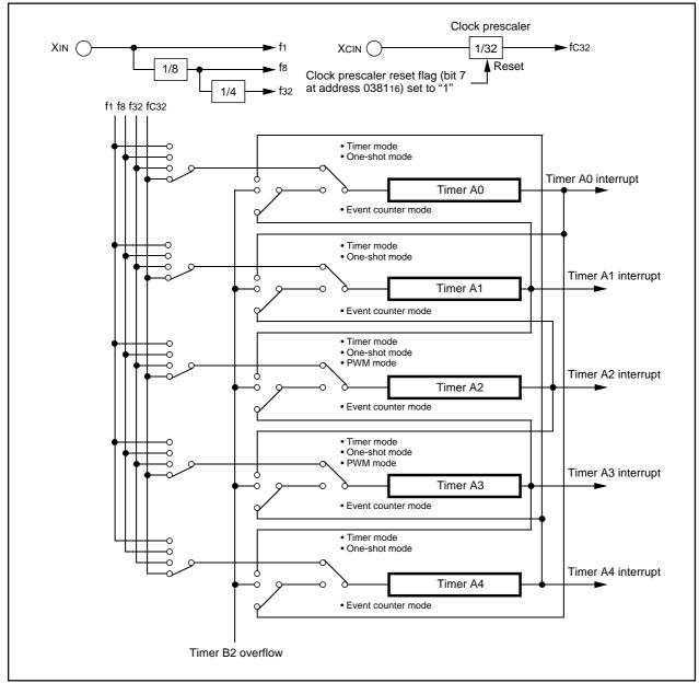
Figure 2.10.1 Timer A block diagram
