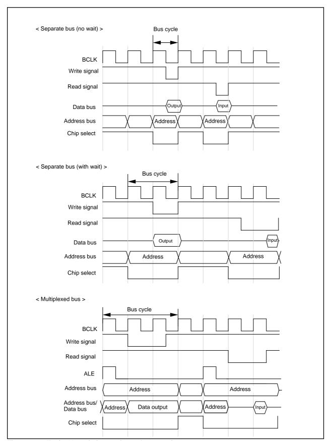
Figure 2.4.8 Typical bus timings using software wait
