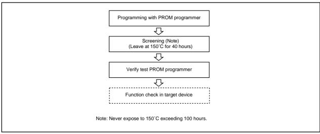
Figure 3.10.1 Programming and test flow for One Time PROM version
