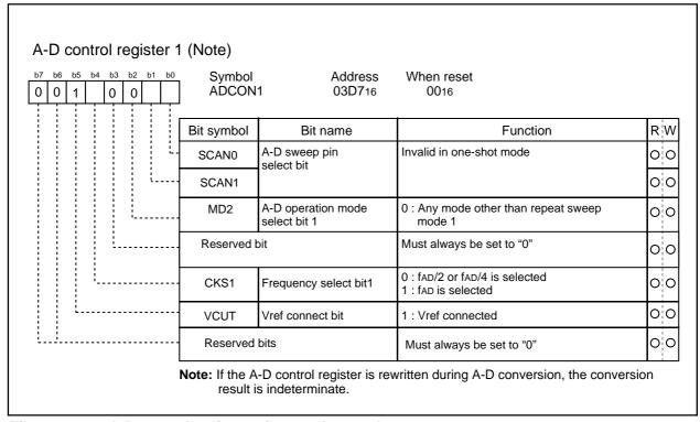
Figure 2.12.7 A-D control register 1 in one-shot mode
