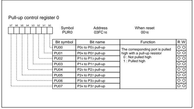
Figure 2.17.15 Pull-up control register 0
