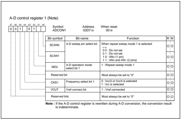
Figure 2.12.15 A-D control register 1 in repeat sweep mode 1
