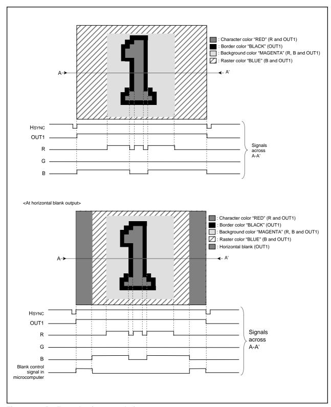
Figure 2.16.52 Example of raster coloring
