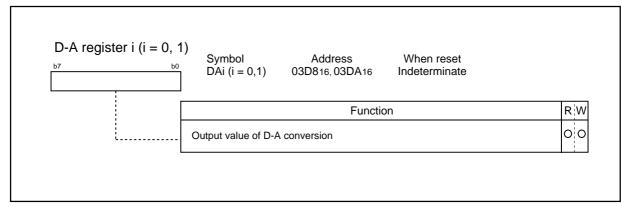
Figure 2.13.3 D-A register i (i = 0 and 1)
