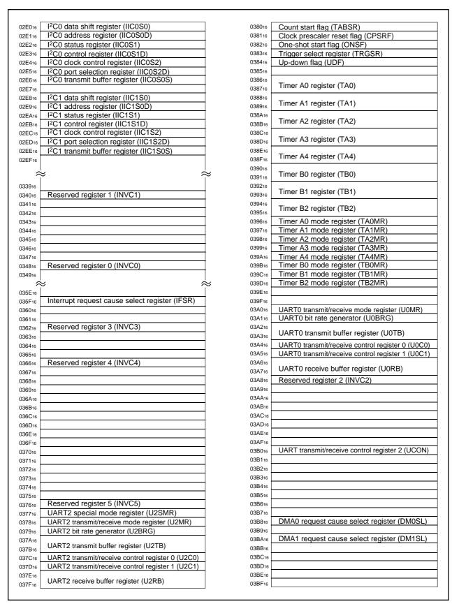
Figure 2.1.4 Location of peripheral unit control registers (3)
