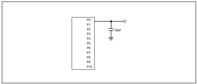
Figure 5.9.1 Port P0 to P10 measurement circuit
