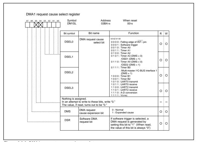
Figure 2.9.3 DMA1 request cause select register
