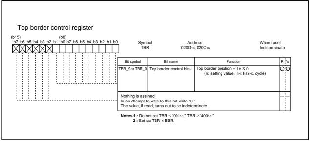
Figure 2.16.47 Top border control register
