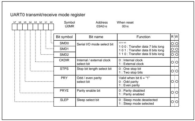
Figure 2.11.21 UART0 transmit/receive mode register in UART mode
