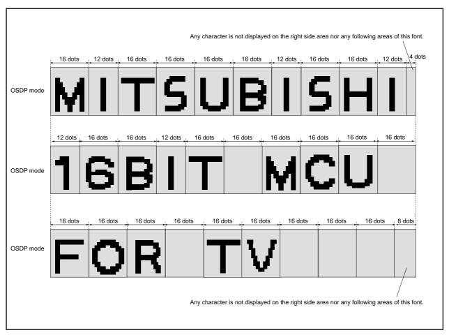
Figure 2.16.39 Display example of OSD mode block
