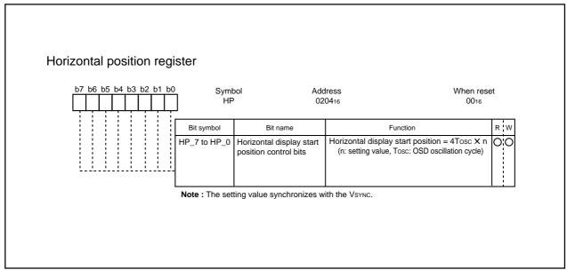
Figure 2.16.11 Horizontal position register
