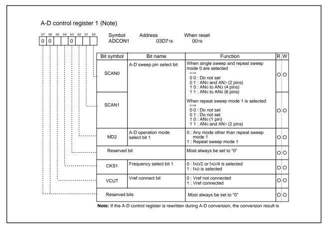
Figure 2.12.3 A-D control register 1
