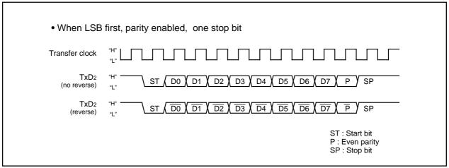
Figure 2.11.24 Timing for switching serial data logic
