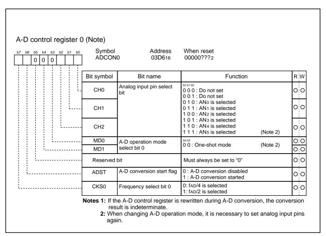
Figure 2.12.6 A-D control register 0 in one-shot mode
