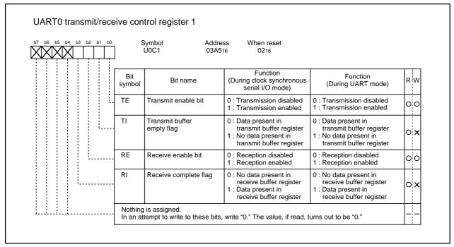
Figure 2.11.11 UART0 transmit/receive control register 1
