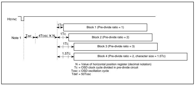
Figure 2.16.12 Notes on horizontal display start position
