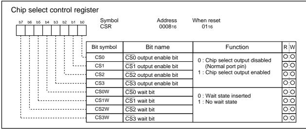
Figure 2.4.4 Chip select control register
