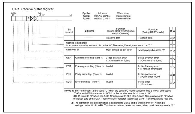
Figure 2.11.5 UARTi receive buffer register (i = 0 and 2)
