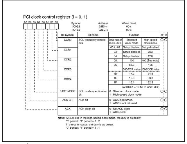
Fig. 2.11.38  $I^2$ Ci clock control register (i = 0, 1)
