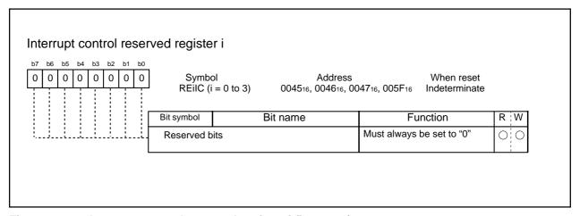
Figure 2.7.10 Interrupt control reserved register i (i = 0 to 3)
