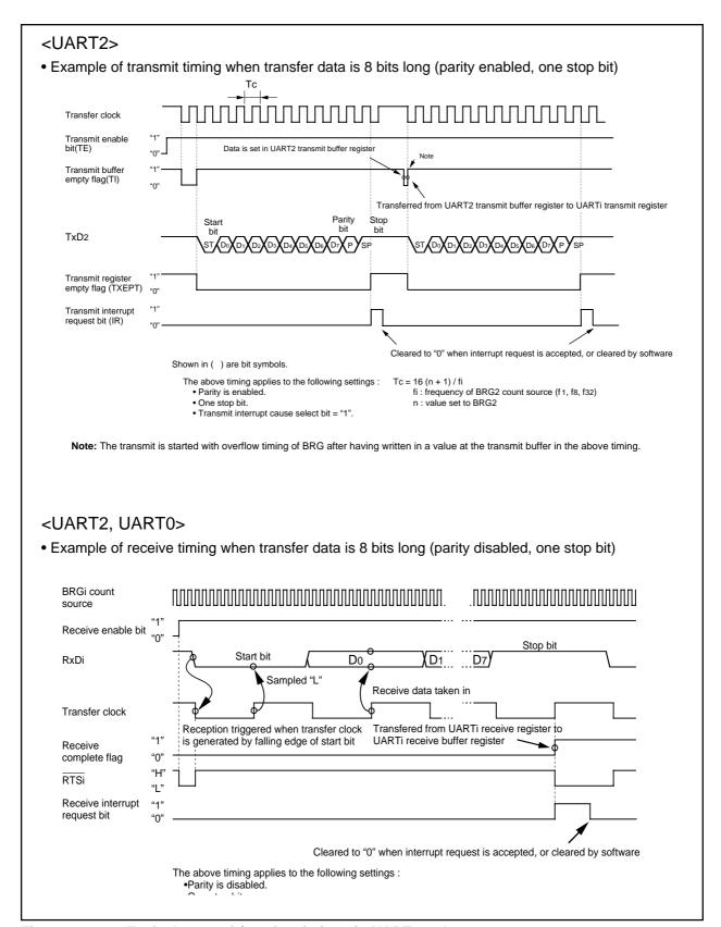
Figure 2.11.23 Typical transmit/receive timings in UART mode
