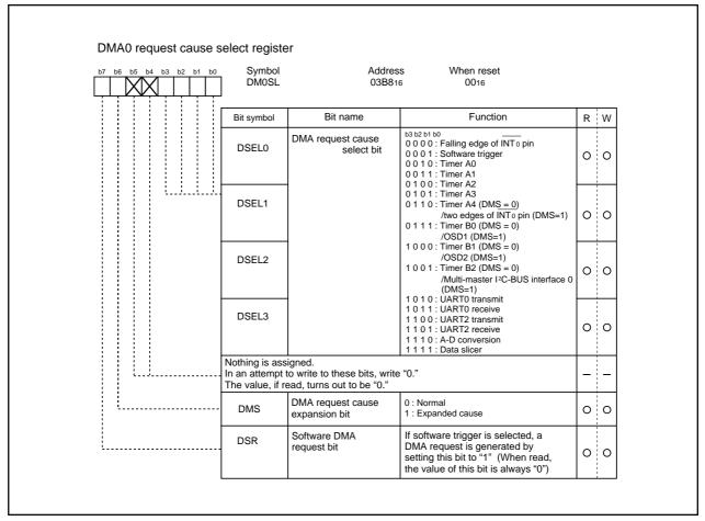
Figure 2.9.2 DMA0 request cause select register
