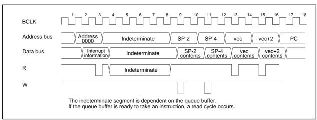
Figure 2.7.5 Time required for executing the interrupt sequence
