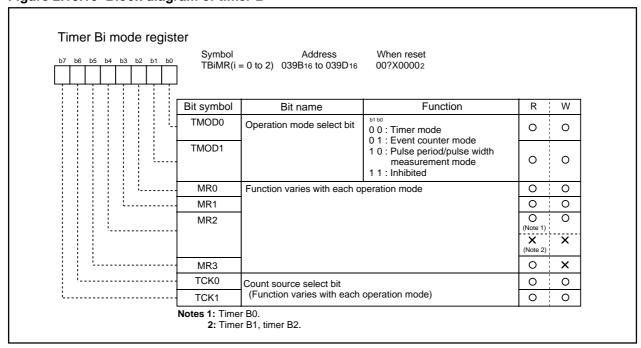
Figure 2.10.17 Timer Bi mode register (i = 0 to 2)
