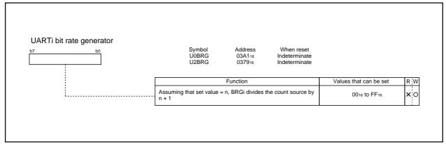
Figure 2.11.6 UARTi bit rate generator (i = 0 and 2)
