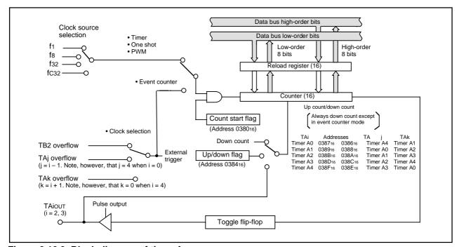
Figure 2.10.3 Block diagram of timer A
