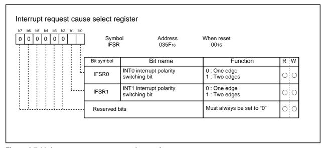
Figure 2.7.11 Interrupt request cause select register
