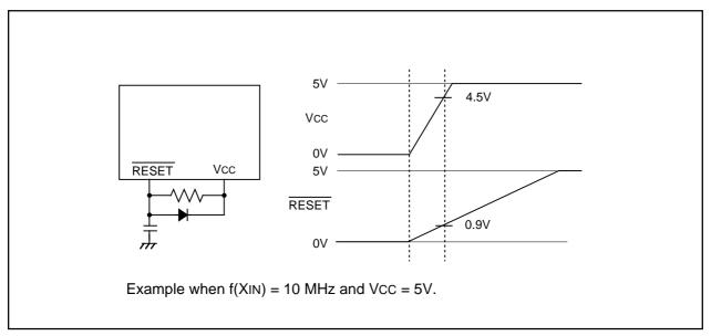
Figure 2.3.1 Example reset circuit
