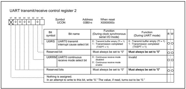
Figure 2.11.13 UART transmit/receive control register 2
