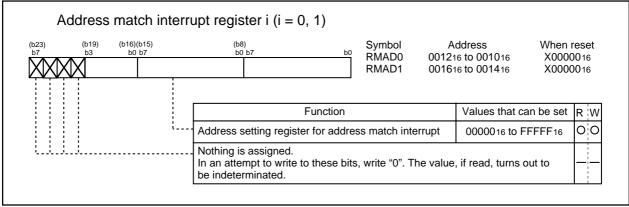
Figure 2.7.13 Address match interrupt register i (i = 0, 1)
