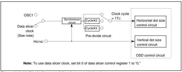
Figure 2.16.13 Block diagram of dot size control circuit
