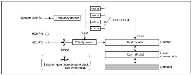
Figure 2.15.2 HSYNC counter block diagram
