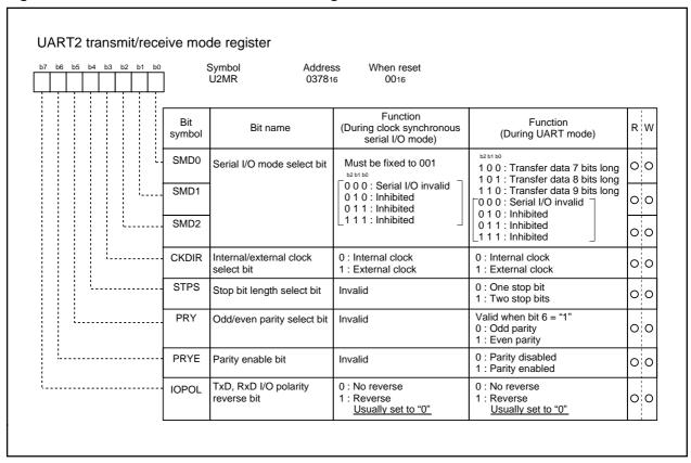
Figure 2.11.8 UART2 transmit/receive mode register
