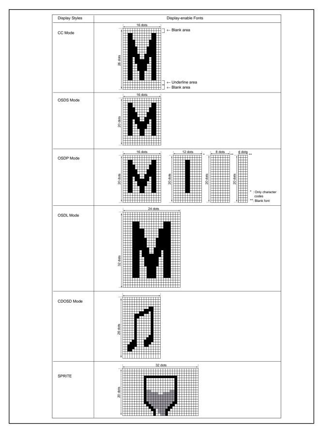
Figure 2.16.1 Display-enable fonts for each display style
