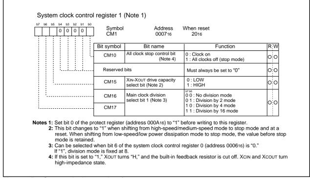
Figure 2.5.6 System clock control register 1
