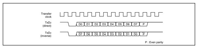
Figure 2.11.29 SIM interface format
