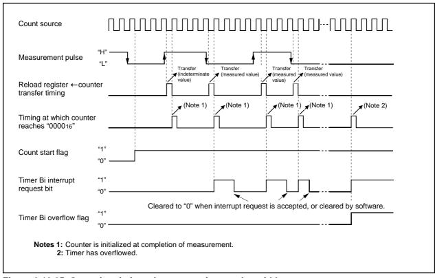
Figure 2.10.25 Operation timing when measuring a pulse width
