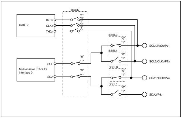
Figure 2.11.31 Serial interface port control
