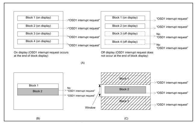
Figure 2.16.40 Note on occurrence of OSD1 interrupt
