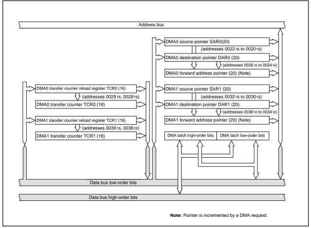
Figure 2.9.1 Block diagram of DMAC
