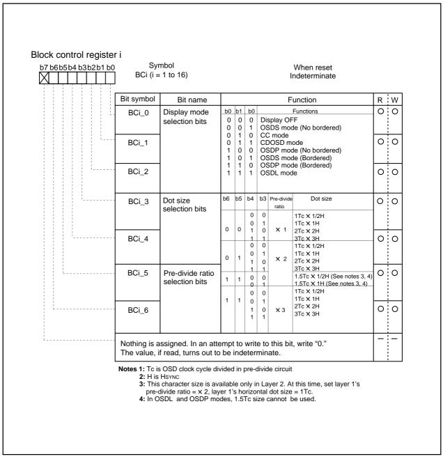
Figure 2.16.4 Block control register i (i = 0 to 16)
