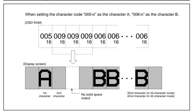
Figure 2.16.38 Display screen example of automatic solid space
