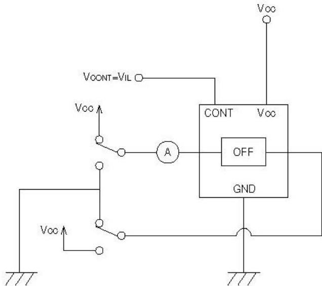
■ Power On Leakage Current
