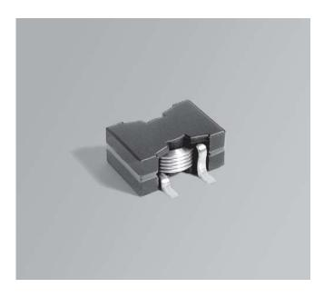
The D1787-AL was developed for use with the National Semiconductor LM5115 Secondary Side Post Regulator Controller and LM5025 Primary Side Controller. This flat wire power inductor offers extremely low dc resistance and very high current ratings (up to 23 Arms). The flat core allows for exceptional heat dissipation and provides an excellent surface for pick and place operation.
