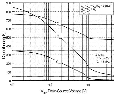
Figure 5. Capacitance Characteristics
