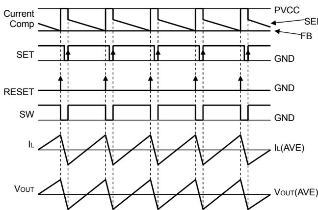
Fig.23 PWM switching timing chart
