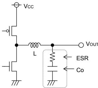
Fig.29 Output capacitor
