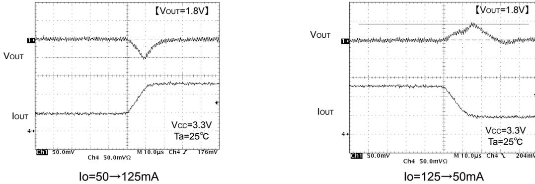
Fig.19 Comparison of transient response
