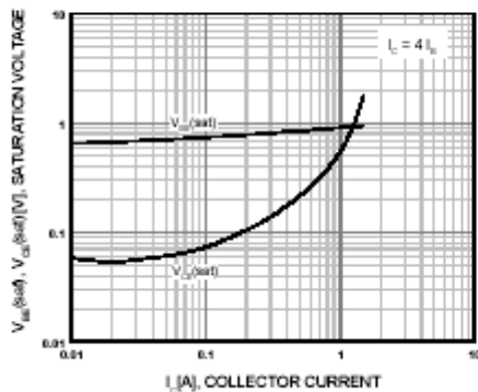
Figure 3. Base-Emitter Saturation Voltage Collector-Emitter Saturation Voltage
