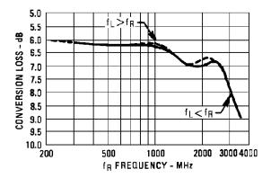
Conversion Loss vs. Input Frequency: Conversion loss of the mixer when used in an SSB system. Data plotted for a  $f_{\parallel}$ of 100 MHz with  $f_1$  at +10 dBm.
