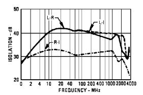
Isolation vs. Frequency: Level of f signal fed through to R- and I-port with respect to the level of the  $\mathbf{f}_{L}$  signal at Lport. R-I Isolation plotted with  $f_{\parallel}$  at 1500 MHz.
