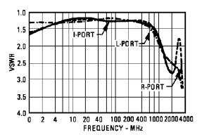
VSWR vs. Frequency: VSWR is the L-, I-, and R-ports in a 50 ohm system with f<sub>I</sub> at +10 dBm. R- and I-port VSWR plotted with f<sub>1</sub> at 1500 MHz.
