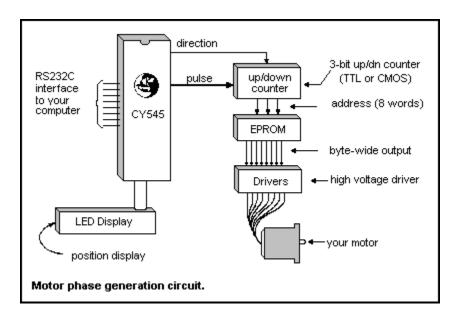
The data outputs from the PROM are then connected to the power driver circuit itself, generating the proper phase patterns for the motor. Note that such a design not only handles motors of various phases, but can also implement stepping schemes such as half-step or quadstep, as well as the standard full-step pattern.
