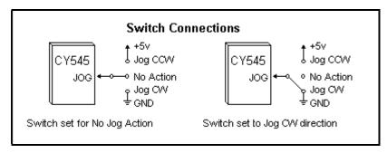
the other side is connected to +5 volts. Jogging is enabled in each direction by pushing the switch from the center position to one side or the other. This is shown in the figure.
