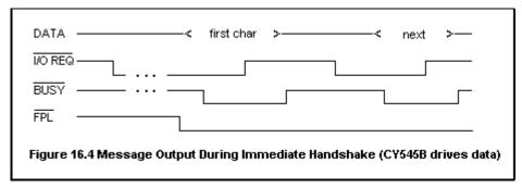
After the CY545B has issued the output message, and FPL is high again, the host may continue with the immediate command handshake, and the CY545B will now accept and execute the immediate command as shown in the second example waveform below. Here, the host does not drive the data bus for the first handshake, and thereby gives the CY545B the "0FFh" first command character prefix. This is followed by the normal first command character.
