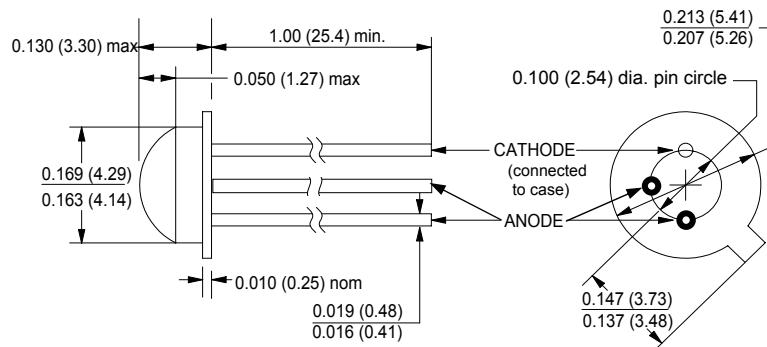
Anode leads must be externally connected together.
