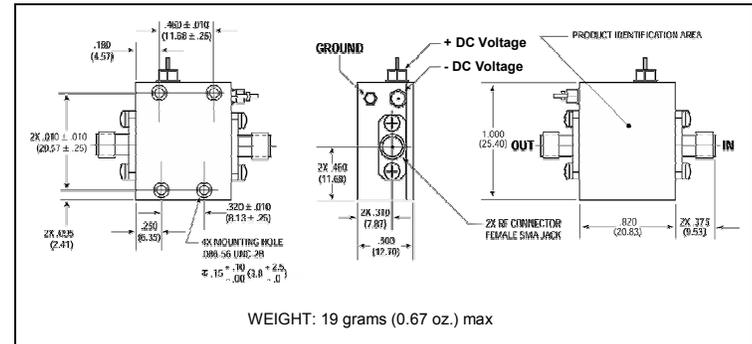
\* Dimensions are inches (millimeters) ±0.015 (0.38) unless otherwise specified.
