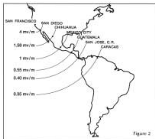
Field strength contour (millivolts/meter) resulting from 516 antenna and 100 kW transmitter located in San Francisco. Data generated by ITS propagation analysis computer program.
