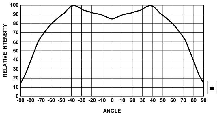
Figure 5d. Relative intensity vs. angle for HSMx-C120.
