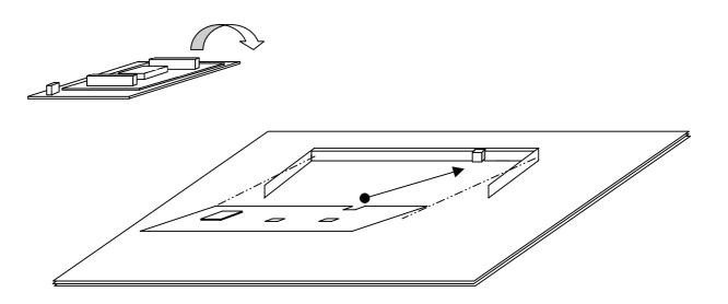
VI) Tilt and slide the SODIMM into the connector Note: The SODIMM can be fitted at one side only (determined by the slot)
