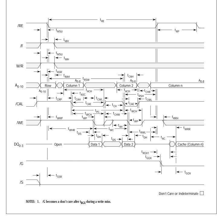
Read/Write During Write Hit Cycle (Can Include Read-Modify-Write)
