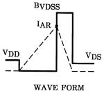
$$\begin{split} R_G &= 25~\Omega \\ V_{DD} &= 25~V,\, L = 165~\mu H \end{split}$$
