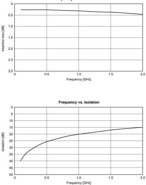
Frequency vs. Insertion loss
