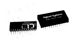
Input Storage Registers — Designed as two 8-Bit segments, the input registers provide data storage when latched, or "transparent" registers when unlatched. Data conversion can now be performed continuously or from stored data — "byte-sized" input segments provide compatibility with most data bus lines.
