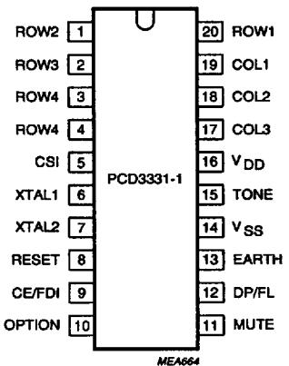
Fig.1 Pin configuration.
