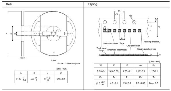
Caution: Insertion direction of device to carrier tape. Marking is on the left bottom side of the cavity to the feeding direction.
