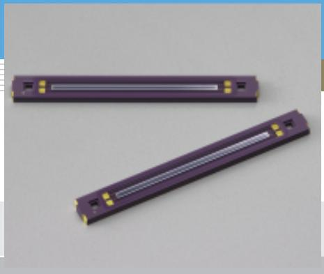
S8543 is a one-dimensional PSD with a long, narrow active area sealed in a surface mountable chip carrier package. The active area of 0.7 x 24 mm delivers excellent position detection characteristics.
