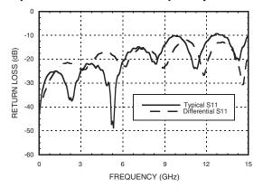
**Output Return Loss vs. Frequency**
