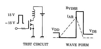
$$\begin{aligned} &R_G = 25~\Omega \\ &V_{DD} = 25~V,~L = 371~\mu H \end{aligned} \qquad EAS = \frac{1}{2} \cdot L \cdot I^2 \cdot \left( \frac{BVDSS}{BVDSS - VDD} \right) \end{aligned}$$
