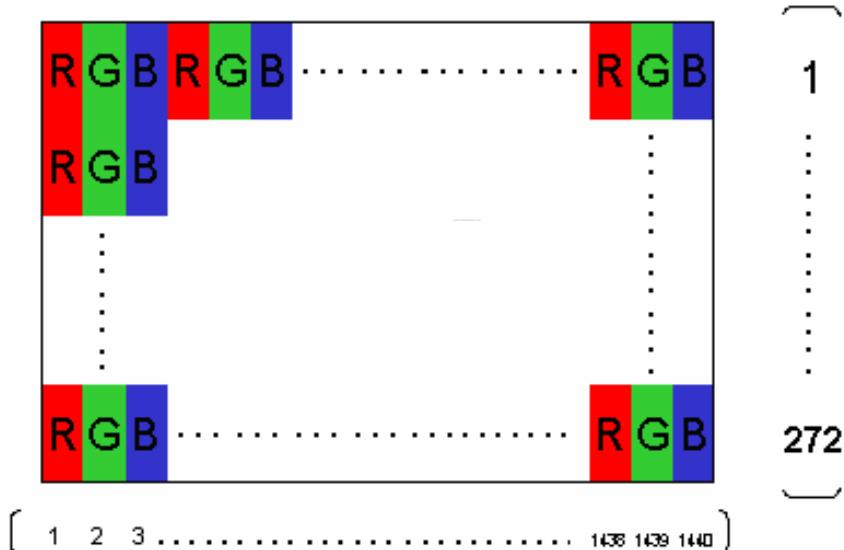
Note 2: Full color display depends on 8-bit data signal (pin 5~28).
