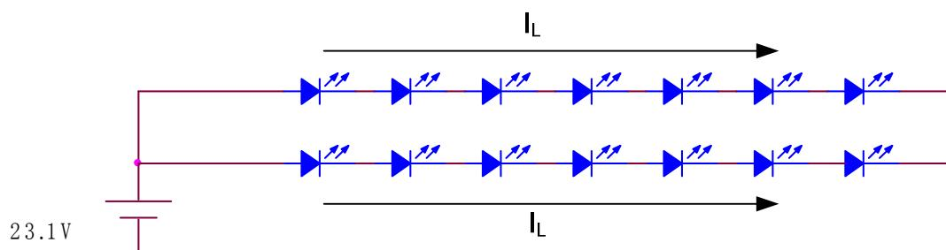
Note 2 :Define “LED Lifetime”: brightness is decreased to 50% of the initial value. LED Lifetime is restricted under normal condition, ambient temperature = 25°C and LED current = 20mA.
