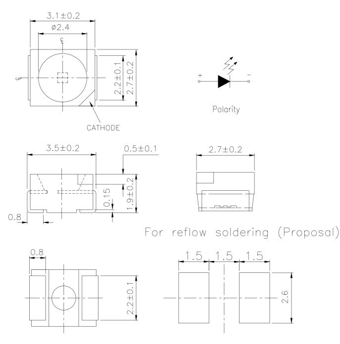
Note: The tolerances unless mentioned is ±0.1mm ;Unit = mm
