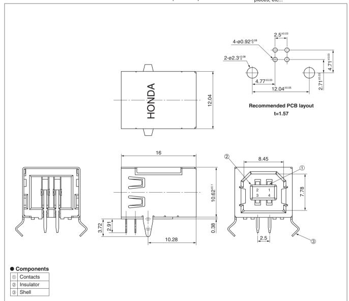
Mating connectors: USB B series connector for cable (USB 2.0 standard)
