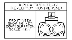
DUPLEX FIBER OPTIC PATCH CORD OPTI-PLUG KEYED "Q" TO SC CONNECTOR CONFIGURATION CUSTOMER DRAWING
