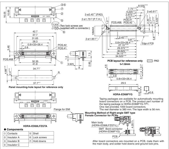
Mating connector: HDRA series IDC type male cable connector, or straddle SMT type male connector on the PCB
