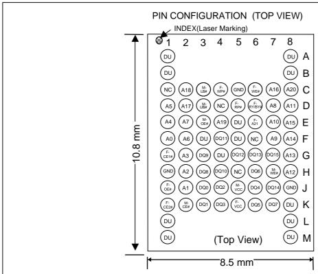
F-VCC : VCC for Flash F-RP# : Reset power down for Flash : VCC for Mobile RAM M-VCC F-WP# : Write protect for Flash : GND for Flash / Mobile RAM **GND** F-RY/BY# : Flash Memory Ready /Busy A0-A20 : Common address for Flash/Mobile RAM M-CE# : Mobile RAM chip enable F-A21 : Address for Flash M-OE# : Output enable for Mobile RAM DQ0-DQ15: Data I/O M-WF# : Write enable for Mobile RAM
